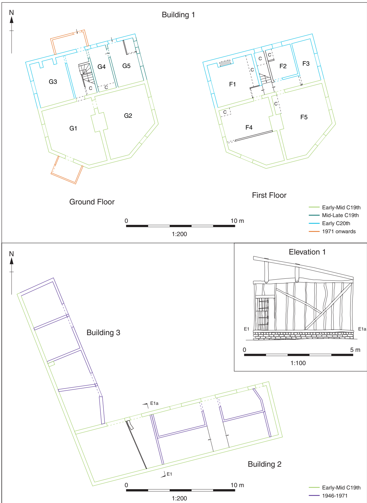
Figure 11: Building 1, ground and first floor plans
