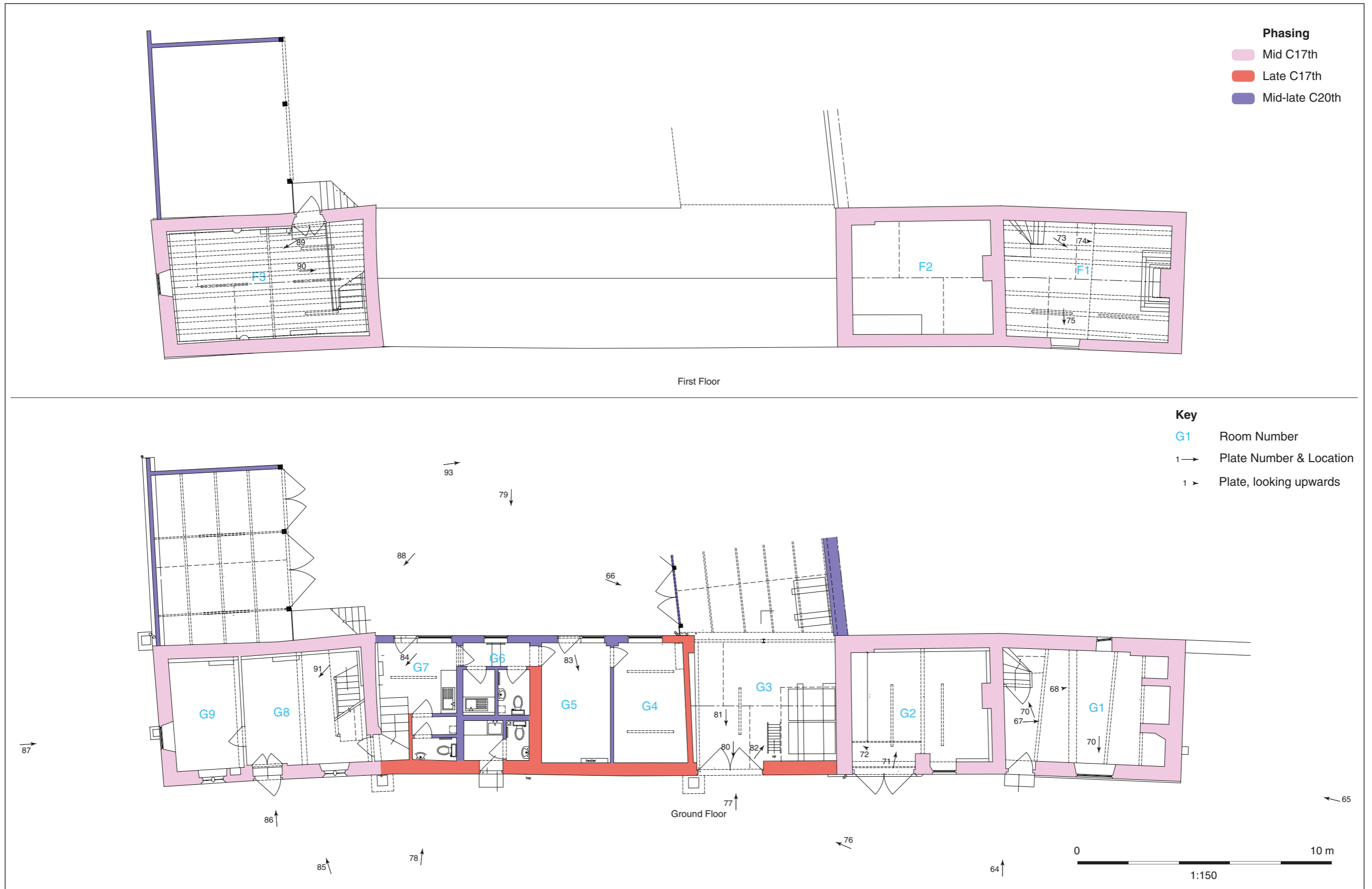
Figure 13: Ground and first floor plans of Buildings 1-3 showing suggested phasing and location of plates referenced in report (from data supplied by client)
