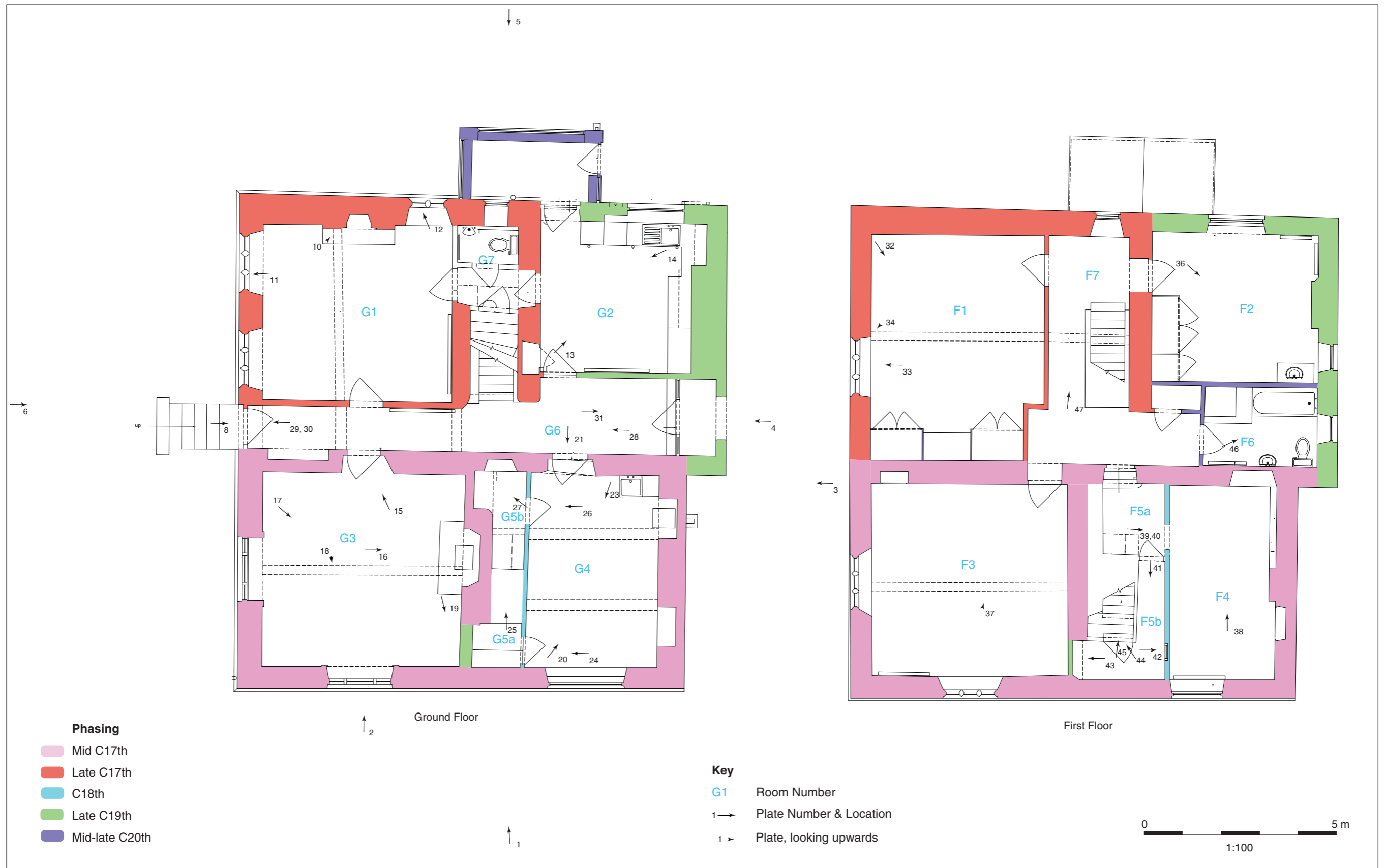
Figure 9: Ground and first floor plans of the farmhouse showing suggested phasing and location of plates referenced in report (from data supplied by client)
