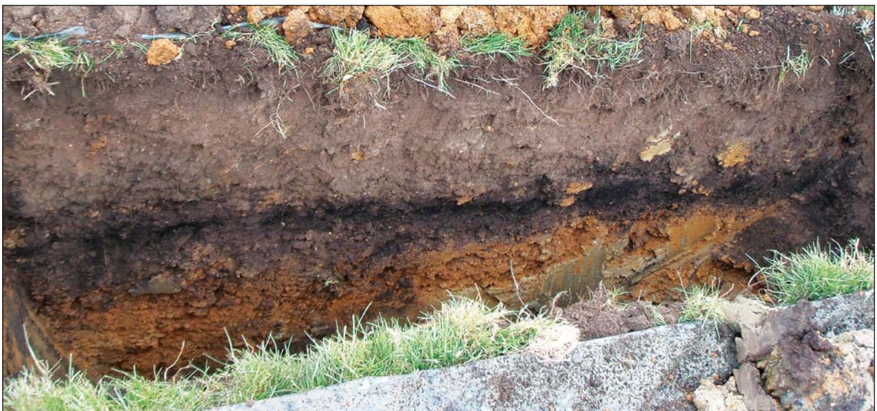
Plate 2: Test pit 223 showing made up ground
