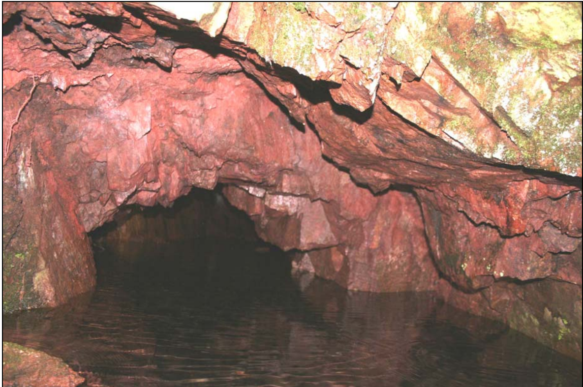
Plate 19: Open drainage adit at the foot of Blea Tarn mine (Site BT24a )
