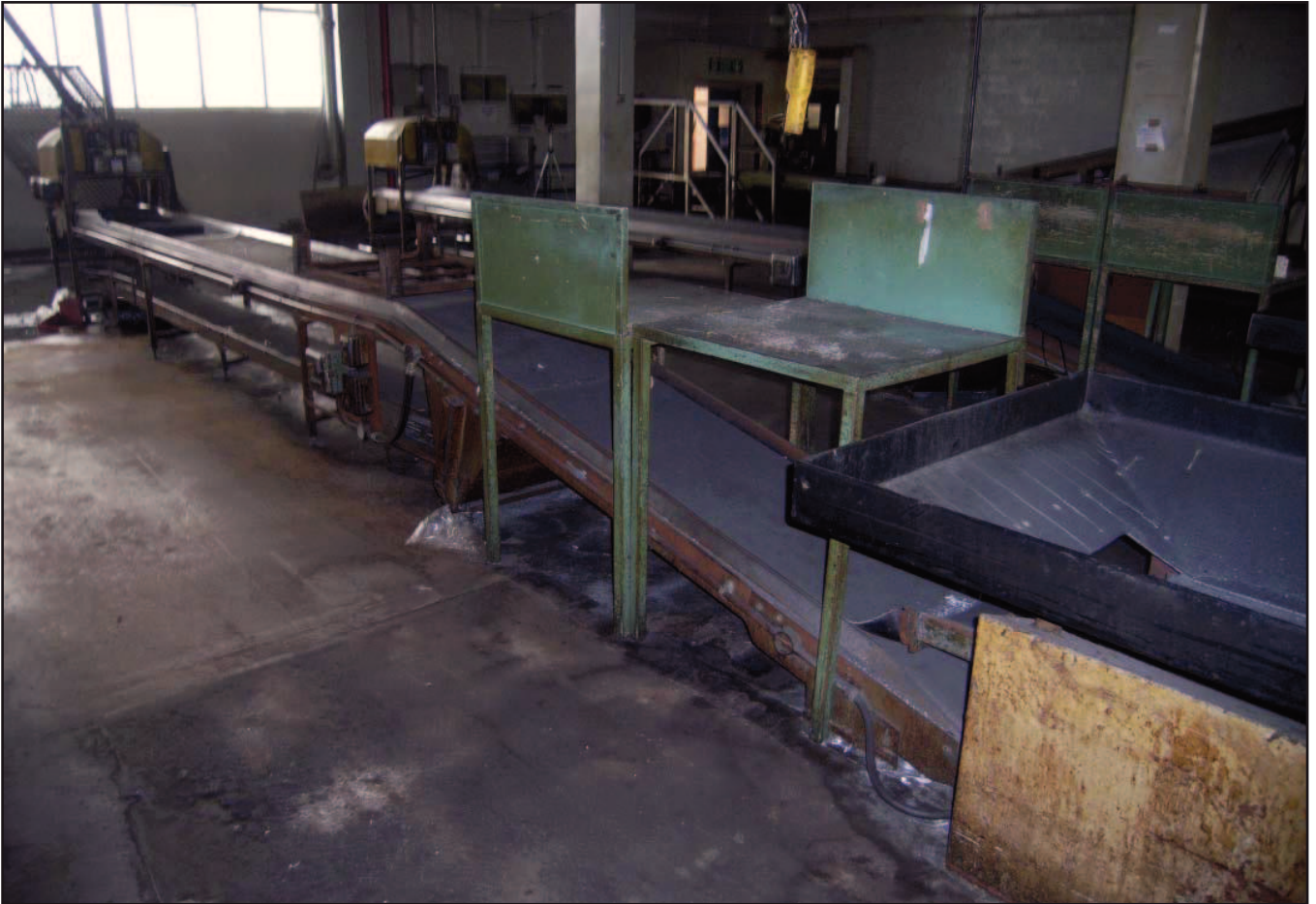
Plate 19: Conveyors in Fetting Dept with Hopper to right.
