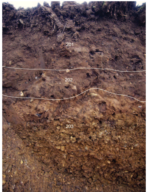
Plate 3: Close up of brickearth/gravel interface in Test Pit 2
