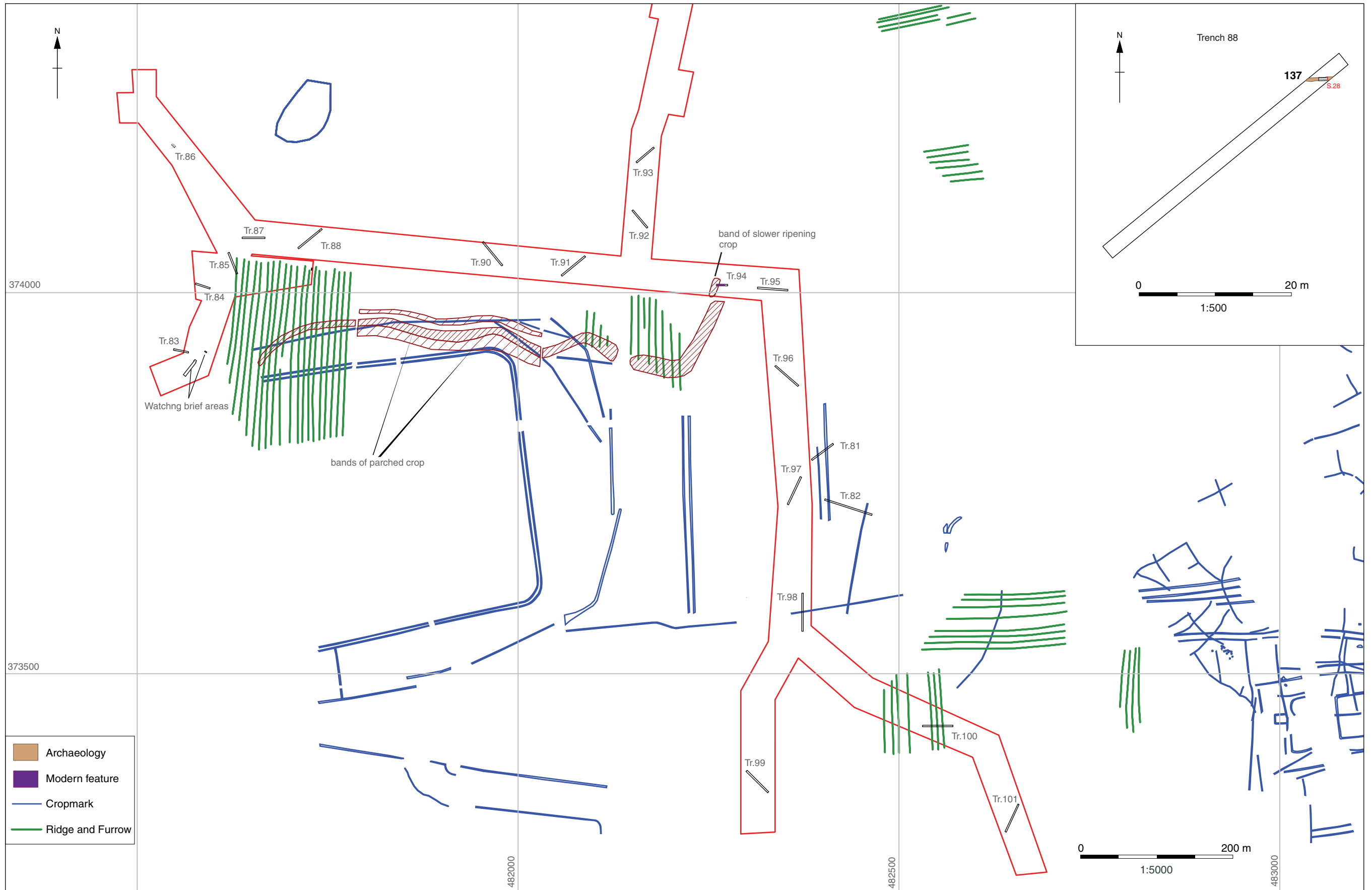
Figure 14: Trench plan, pipeline route, pumping station and compound area in relation to mapped cropmark features
