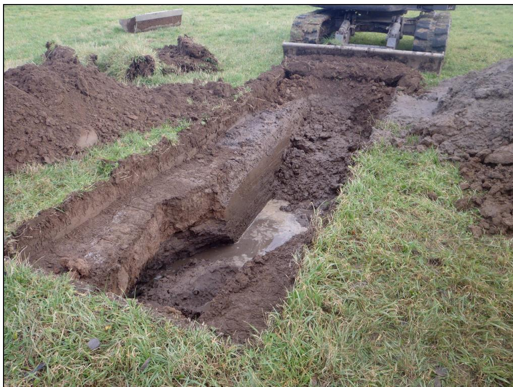
*Plate 3 An example of edge collapse due to adverse ground conditions in TP011. Viewed facing north-east.*
