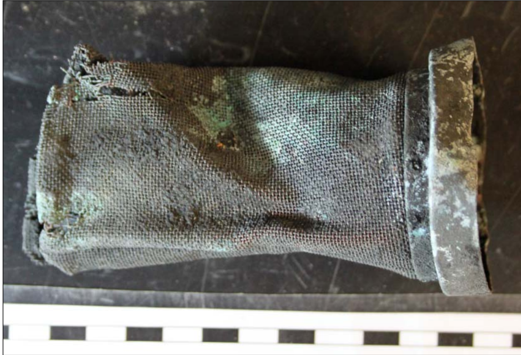
Plate 53: Outer gauze of a miner's safety lamp
