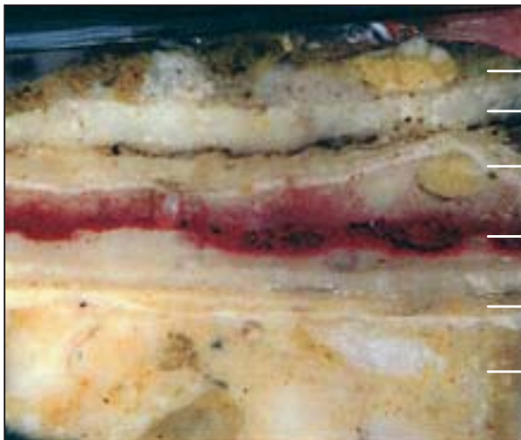
Medieval DIY! - A close-up photograph of the layers of paint and whitewash on a fragment of wall plaster from the guest hall.
