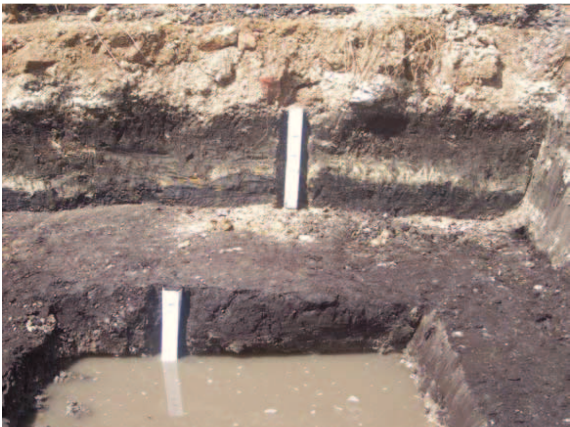
Plate 4: Monolith sampling of alluvial/peat sequence, TP01
