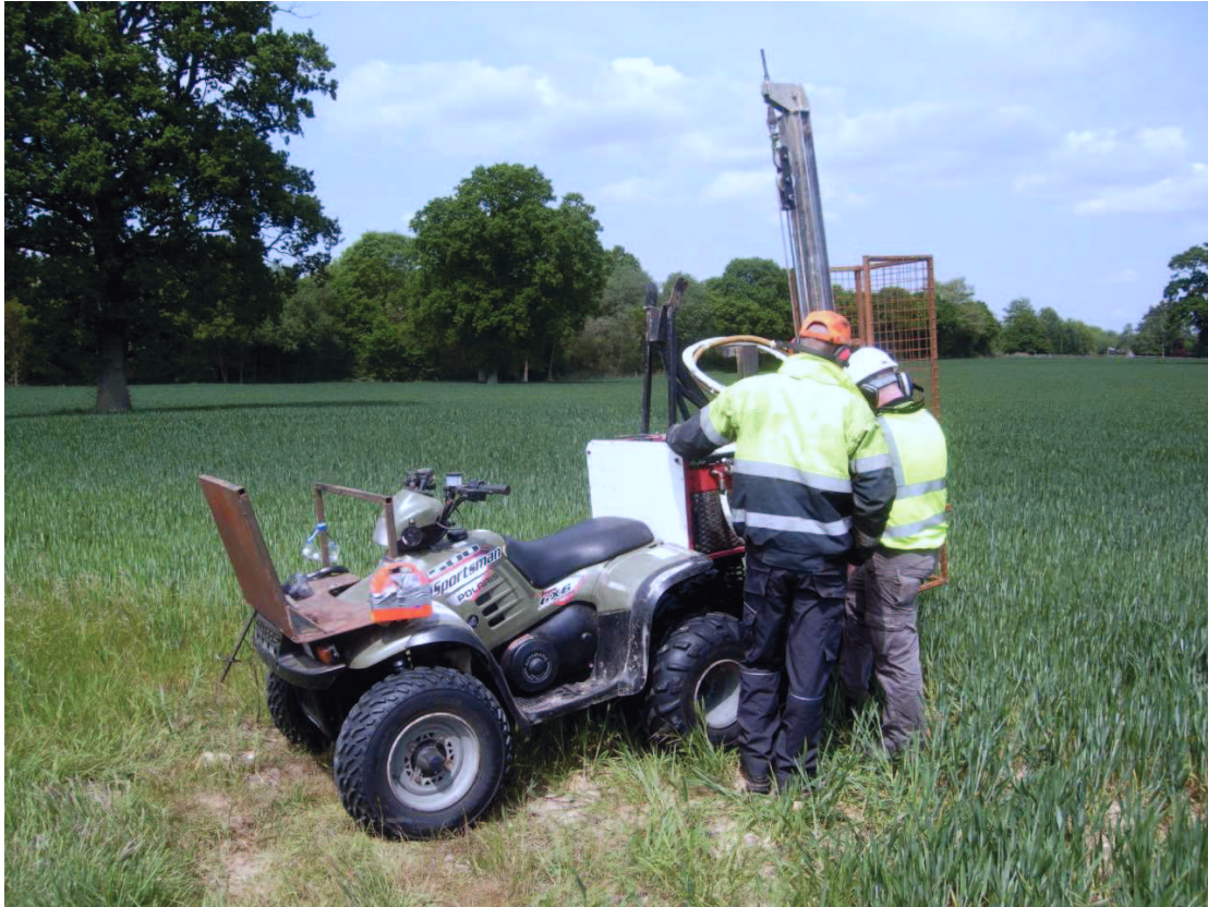
Plate 3: Auger drilling at location TP2 in preparation for the seismic charge
