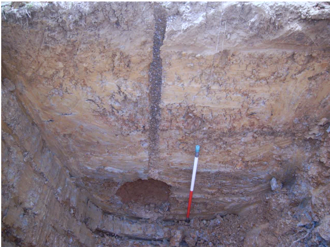
Plate 2: Section of Trial Pit 1 showing the blast crater of a 200g explosive charge
