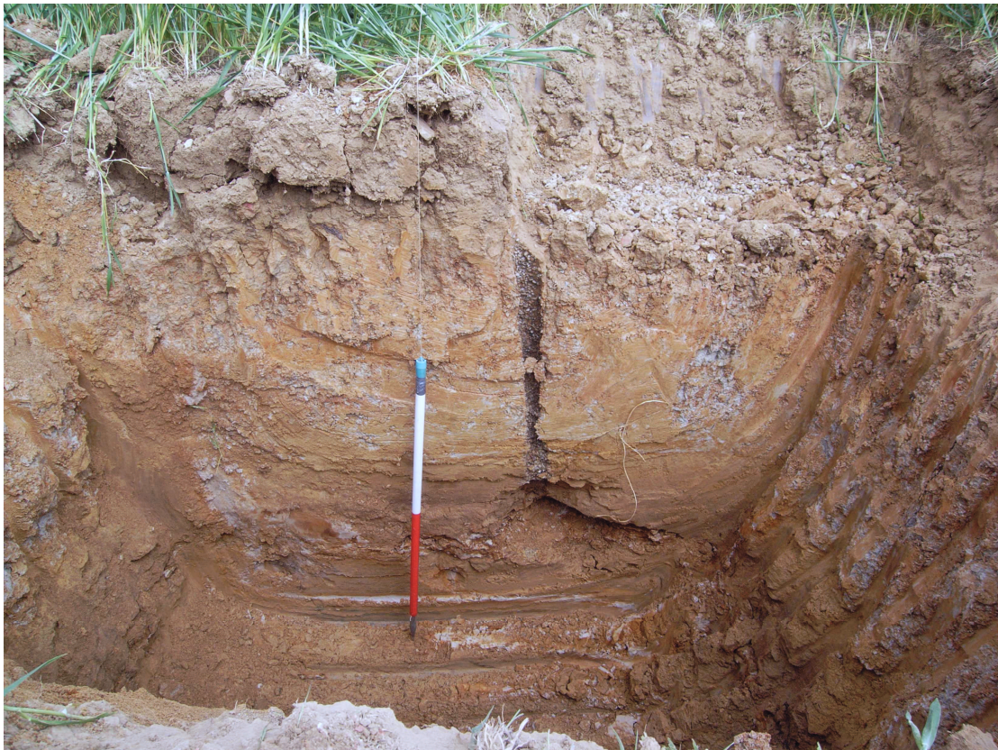
Plate 4: Section of Trial Pit 2 showing the blast crater of a 200g explosive charge
