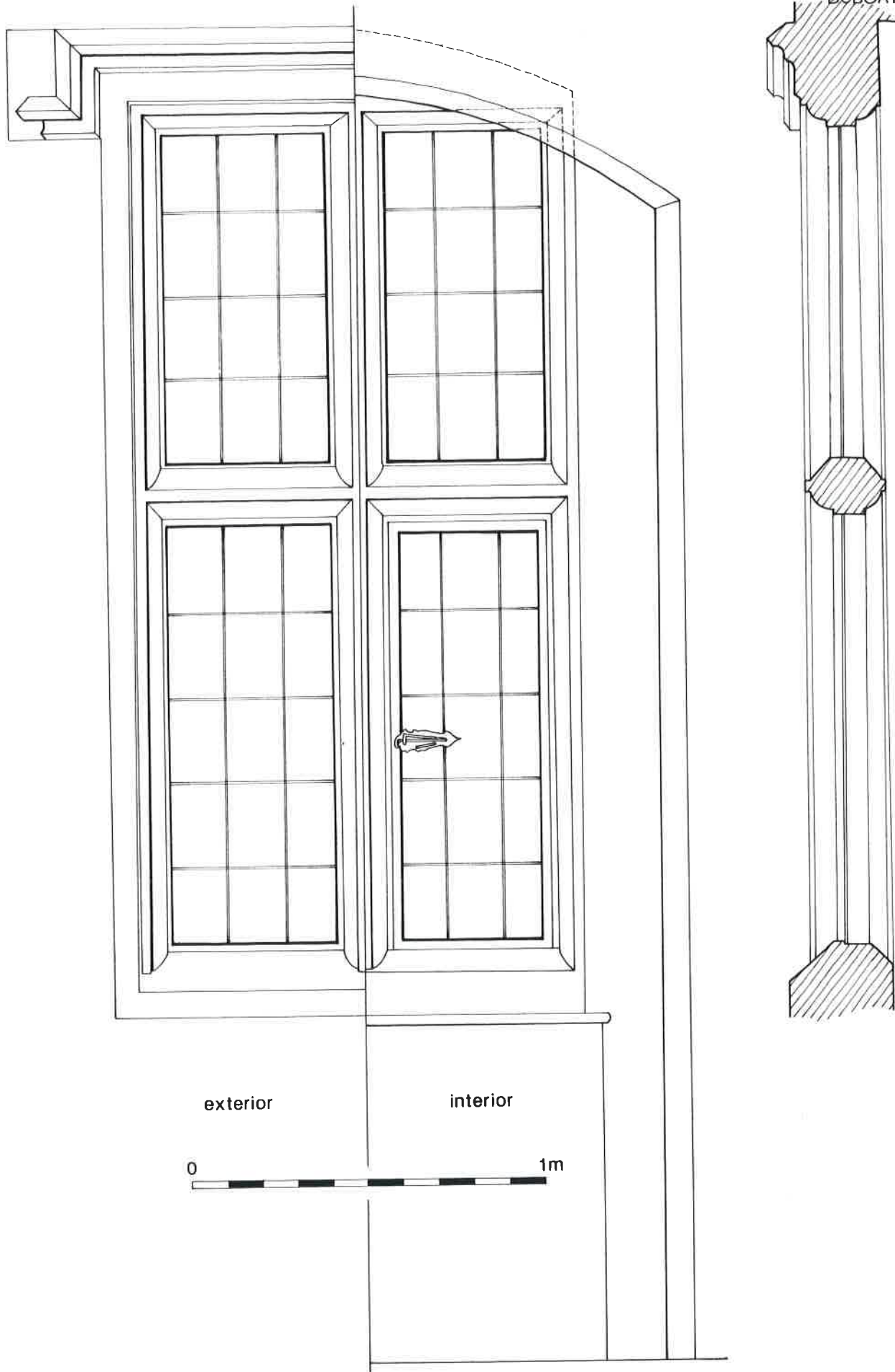
Figure 21: Window detail ; 2F/01, south-west wall
