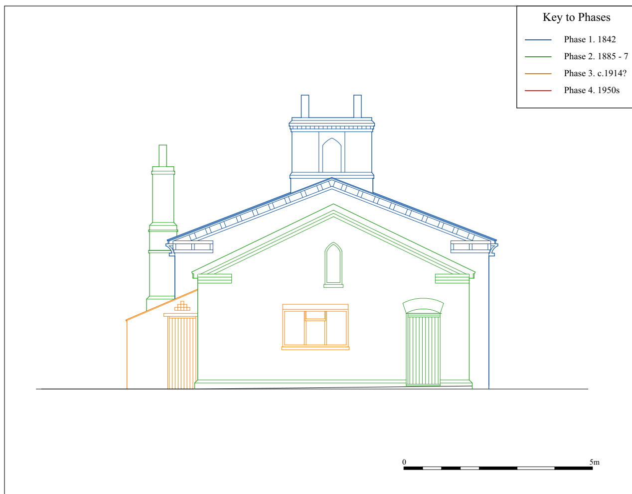
Figure 3: East-facing elevation (1:100), with phasing, from data supplied by client
