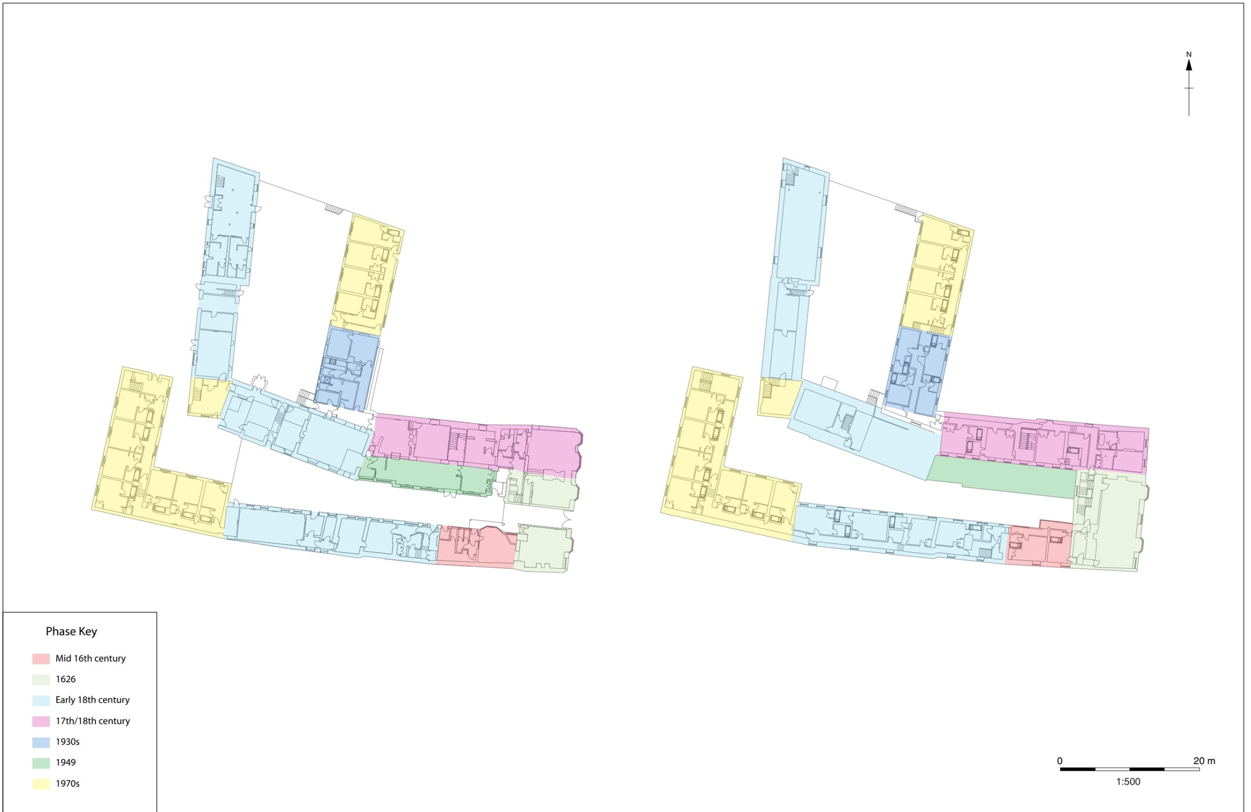
Figure 3: Ground and first floor plans of the Talbot Hotel with suggested phasing (data supplied by client)
