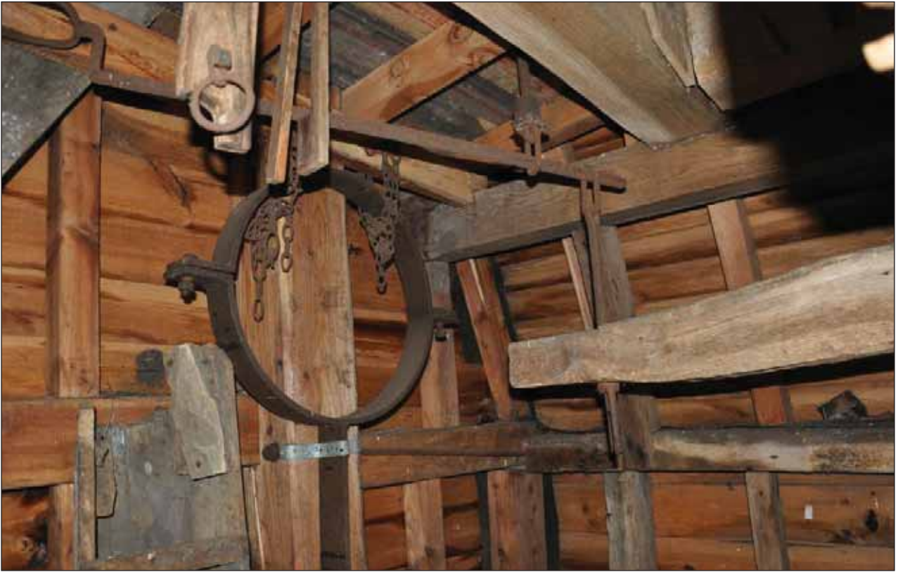
Plate 11: Tentering gear for Lag Governor. wooden grain
