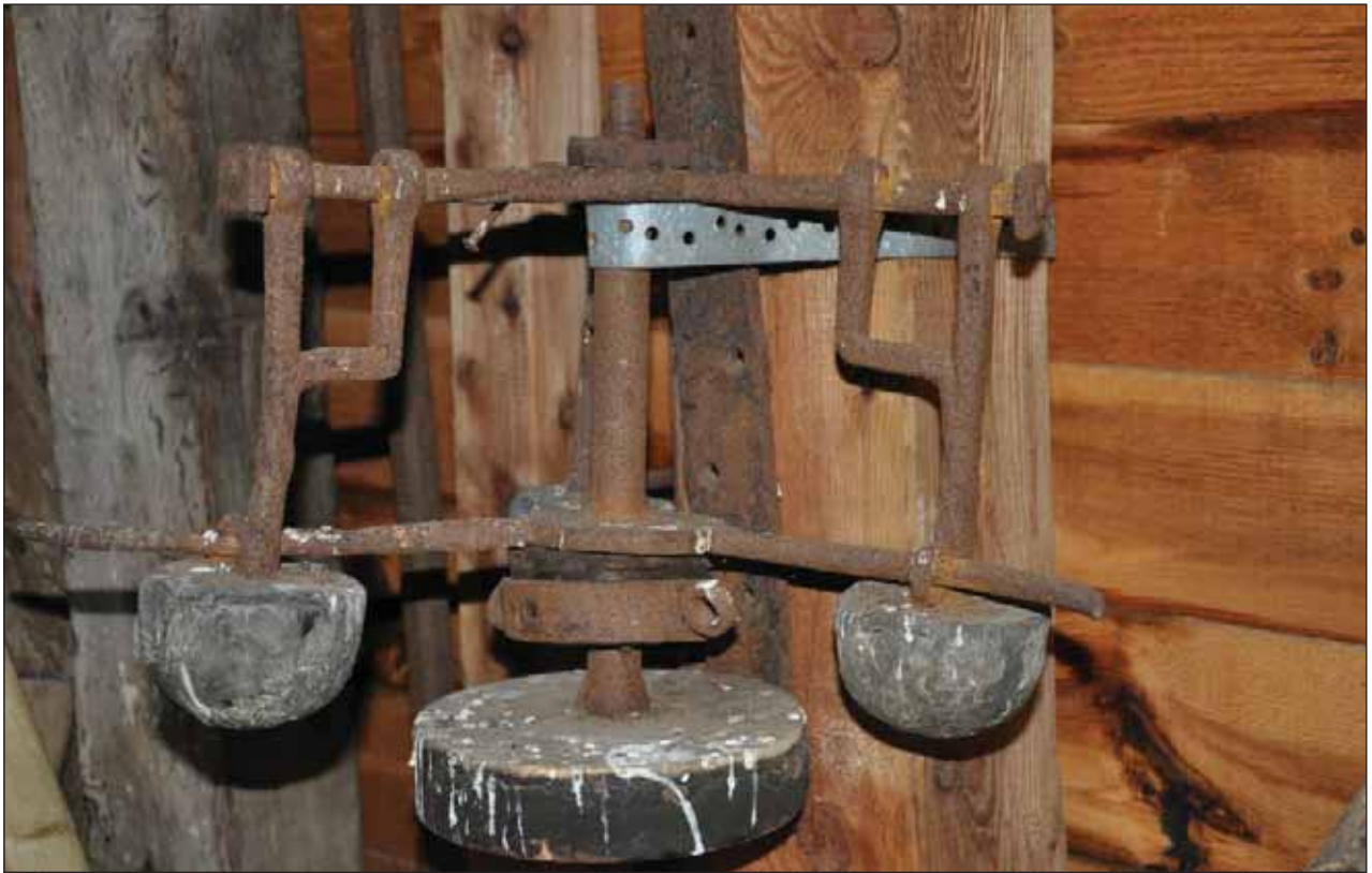
Plate 17: Lag Governor - as DSC 6005 - side view.
