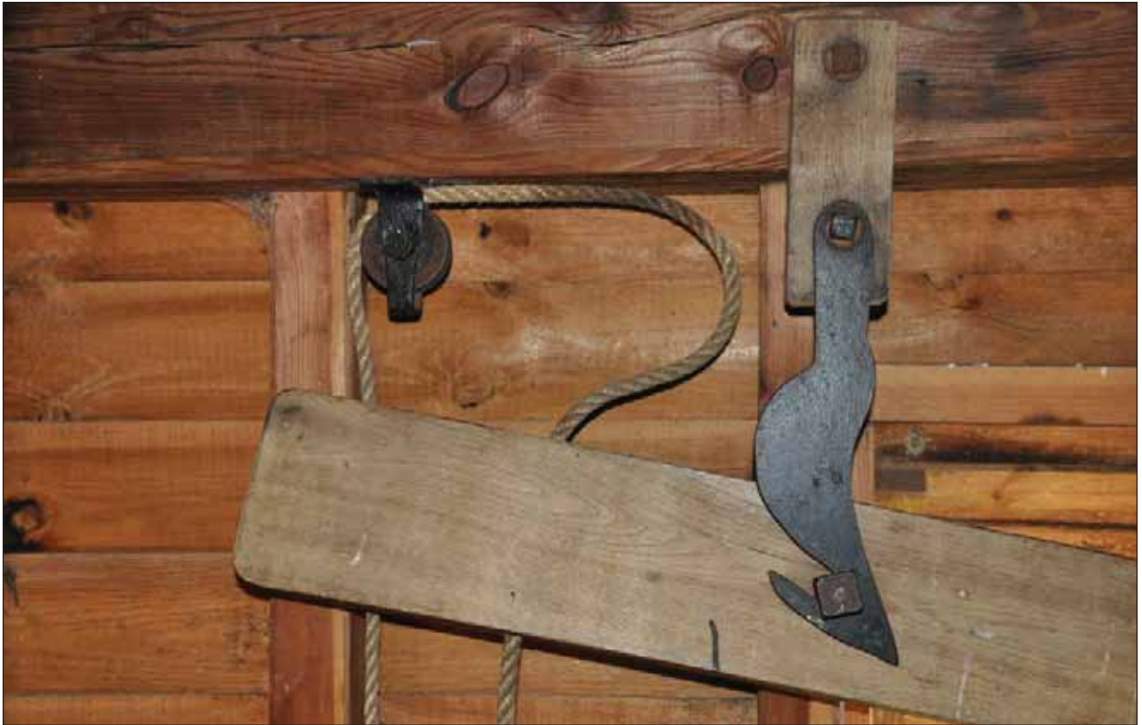
Plate 51: Metal hook to hold brake-lever in “brake not engaged” position.
