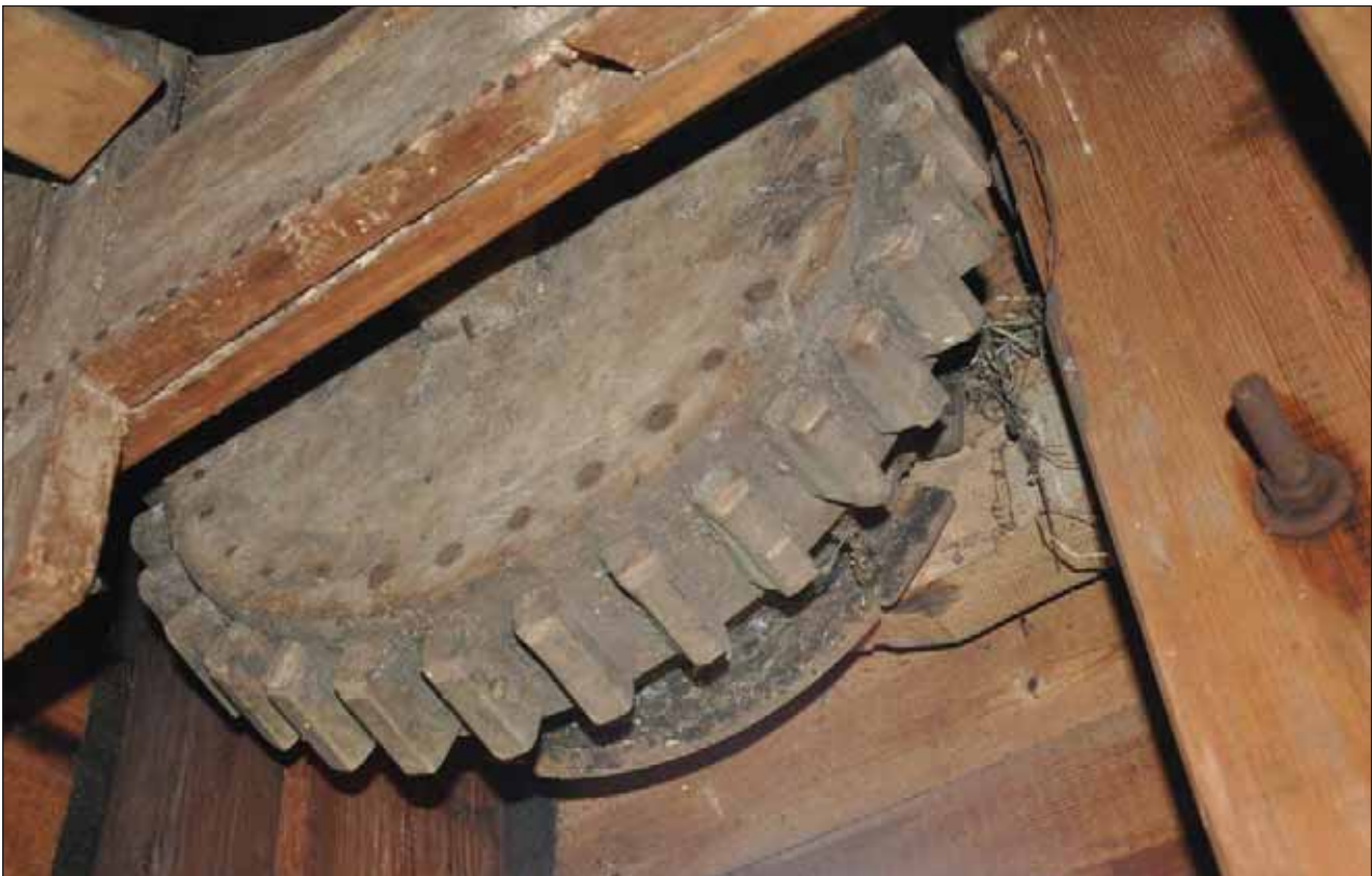
Plate 30: Belt wheel and drive cog to power the flour bolter.
