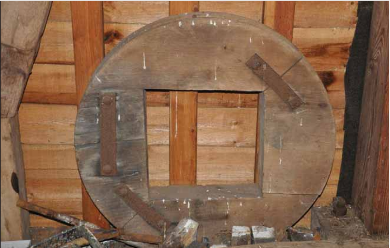
Plate 31: Hopper to feed grain into centre of top of a millstone.
