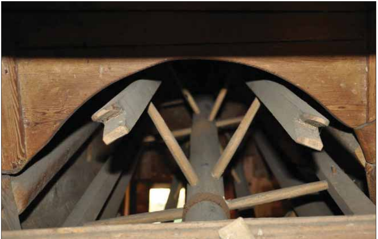
Plate 36: Central spindle and radial arms of bolter
