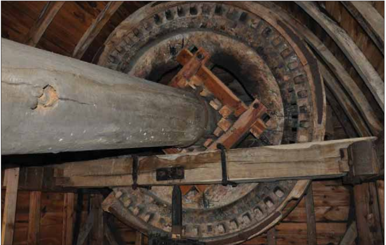
Plate 47: Brakewheel , windshaft and Sprattlebeam.
