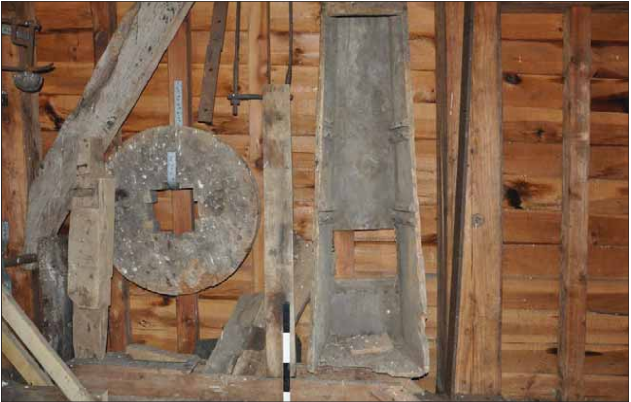
Plate 7: Belt pulley wooden wheel for sack hoist;
