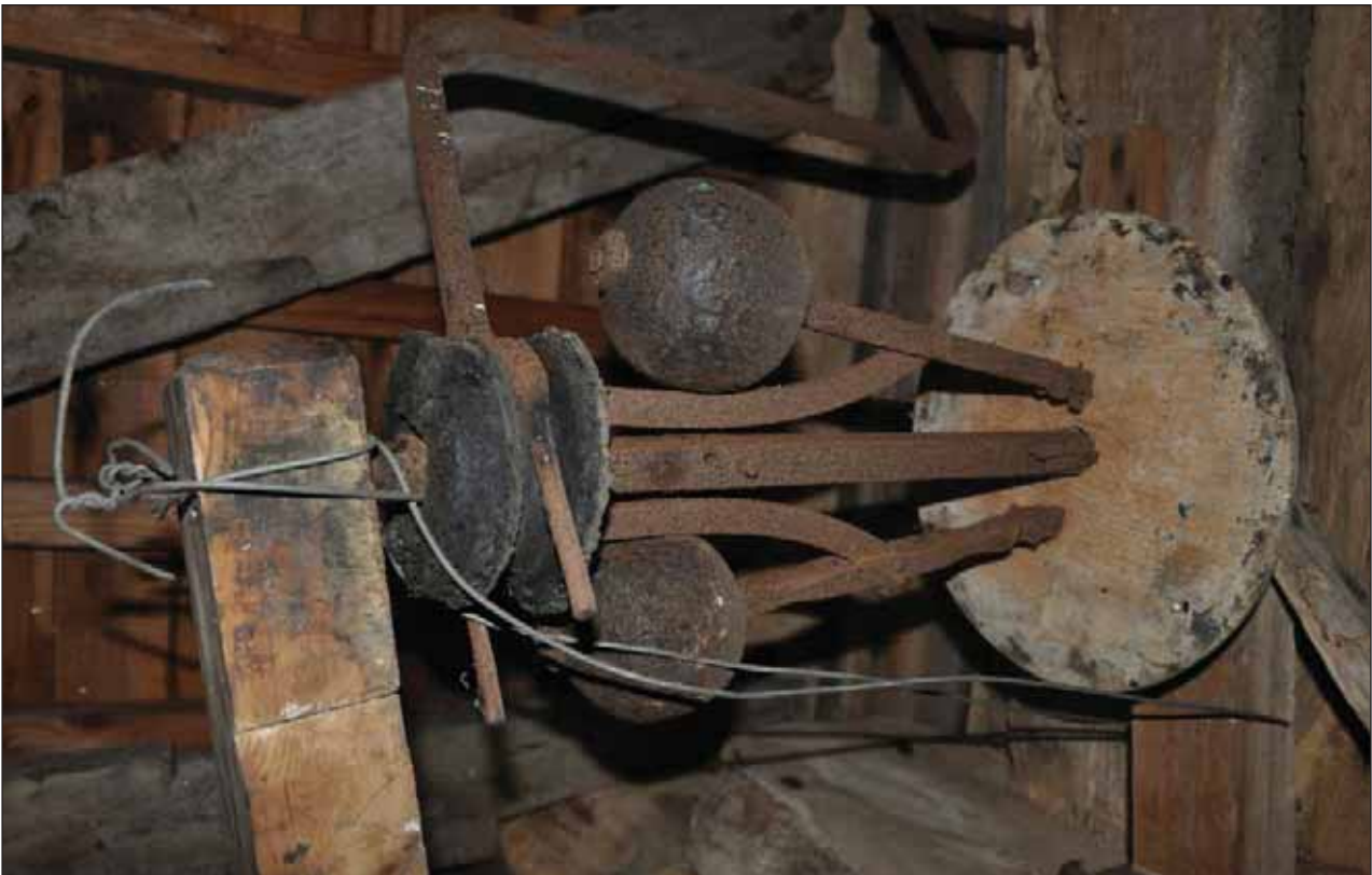
Plate 24: Governor used on front set of stones.
