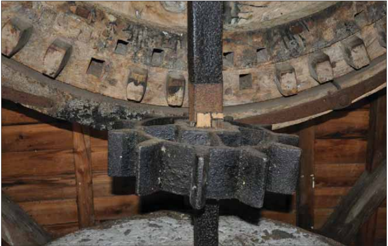
Plate 41: Stone nut over front stones and lower edge of brake wheel and brake rim.
