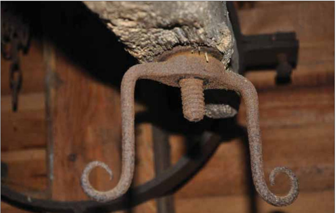
Plate 12: Tentering screw on tentering gear.
