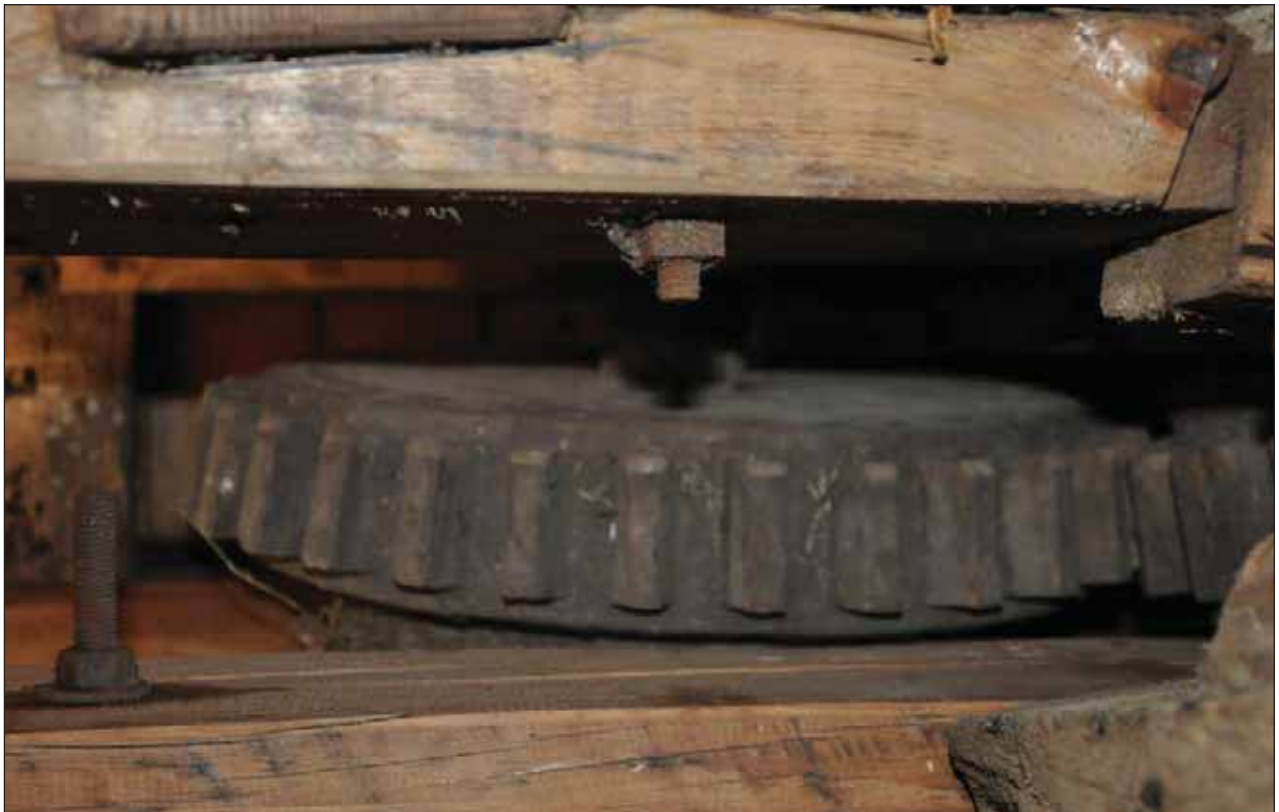
Plate 38: Drive cog to engage with cog on end of bolter spindle.
