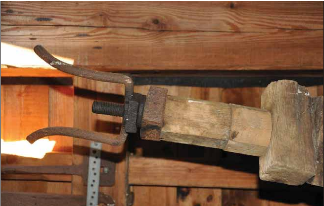
Plate 23: Tentering screw for tentering gear of governor on front stones.
