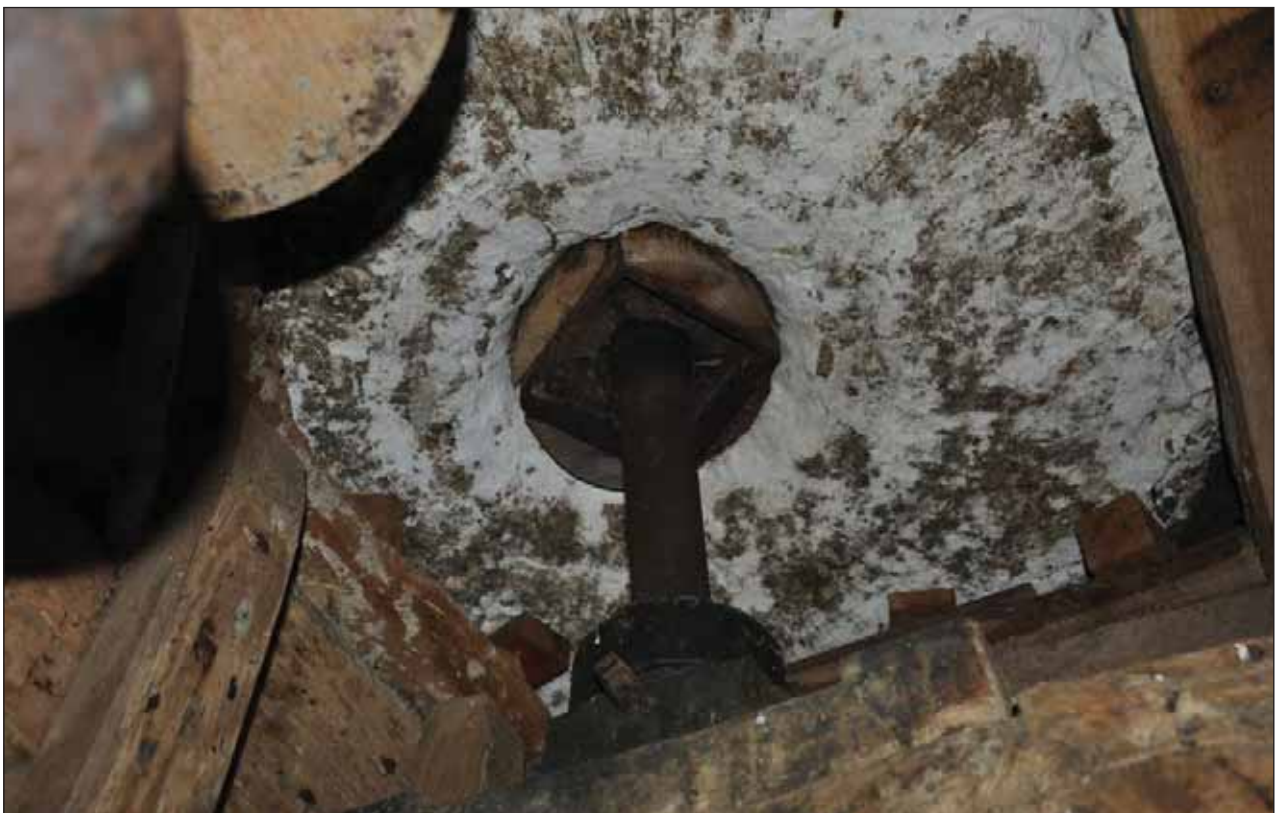
Plate 26: Stone spindle under front set of stones.
