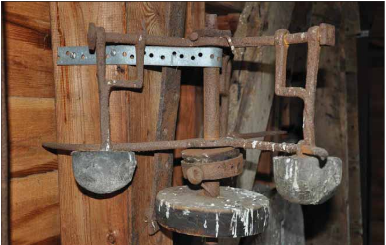
Plate 18: Lag Governor - as DSC 6005 - side view
