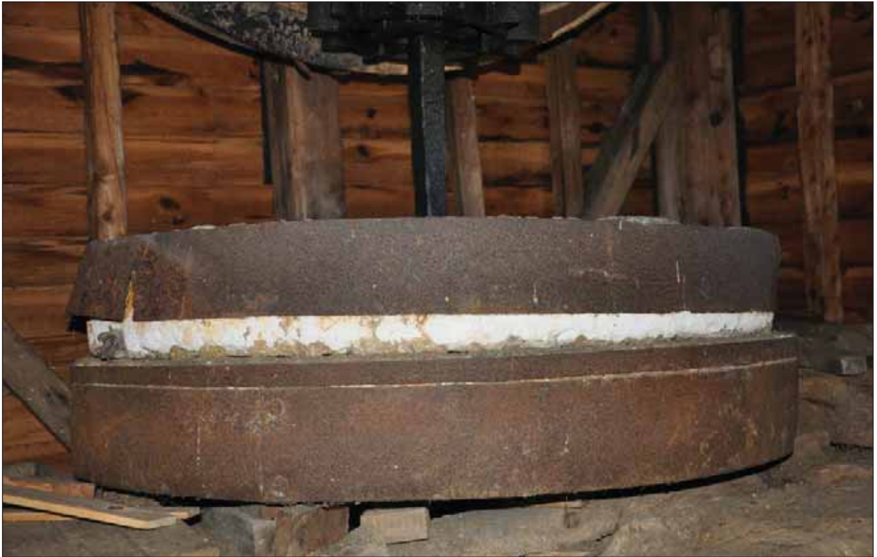
Plate 43: Front "pair" of millstones - lateral view.
