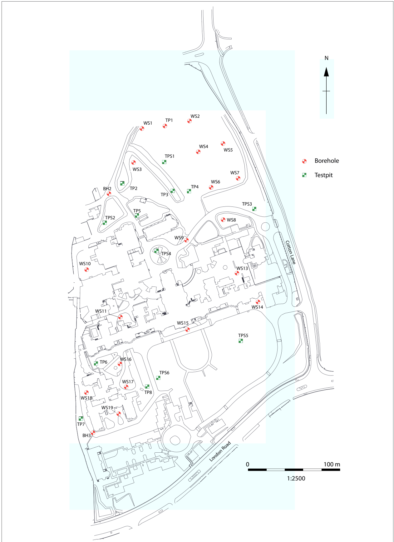
Figure 2: Plan of site and geotechnical investigations
