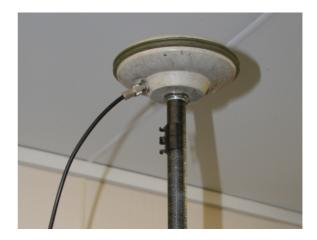
The aerial screws onto the top of the backpack – the port below which there is a cable
