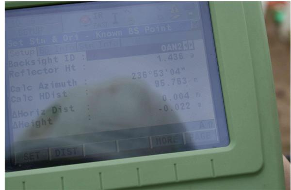
The given example (above) is too large a residual. In this case the station height, levelling for both station has to be re-checked!
