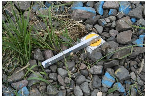
Spread the legs over the point so that the plate is level, and the hole of the screw over the point. Please note that the plate does not have an actual level, but that this is only for initial judgement by the eye.
