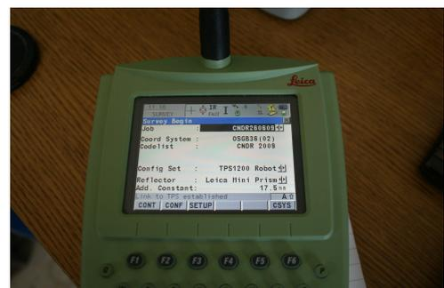
Choose the method “Known BS point” and the Station Coord. “From Fixpoint Job” - this is the job from which you retrieve the station information. The station information for your job should be stored on a job called ‘Project\_Control’. Type in the instrument height just measured off the Total Station after writing it into the survey book. Press cont.
