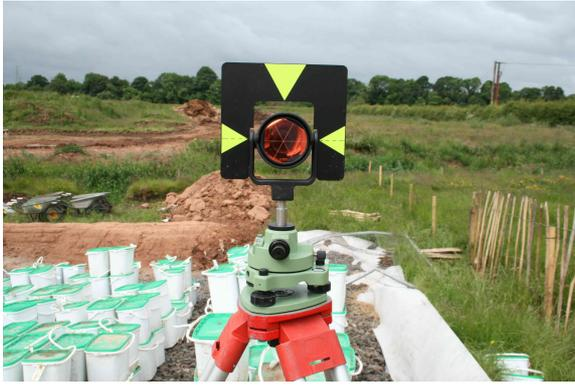
Open the orange box, and remove the circular prism. Turn the prism to face the Total Station on the station point.
