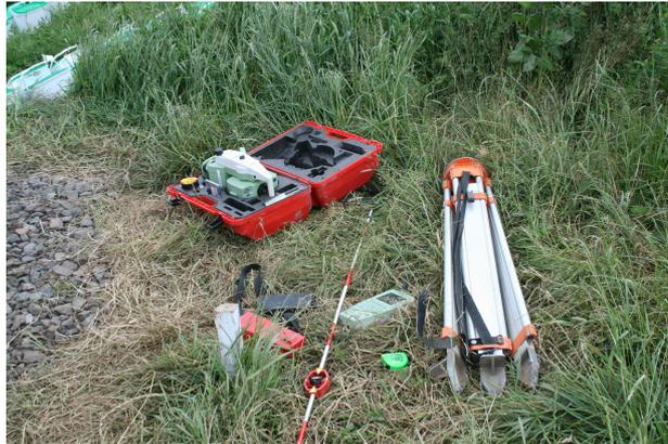
**Step 1:** Go to *the station point* to set up the Total Station
