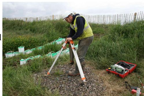
Press the pointy ends of the legs firmly into the ground, ensuring the tripod stays level
