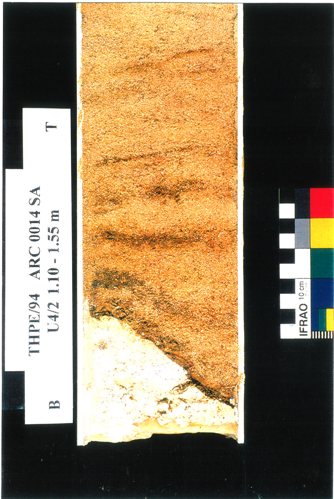
Plate 9. U4 2 core at 1.10-1.55m below ground surface (lower part), borehole ARC 0014 SA, showing sharp contact between the sands and underlying chalk bedrock.
