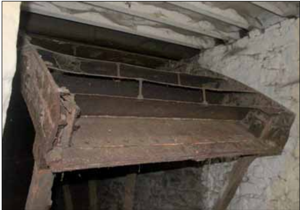
Plate 71: Detail of buckets and spoke sockets
