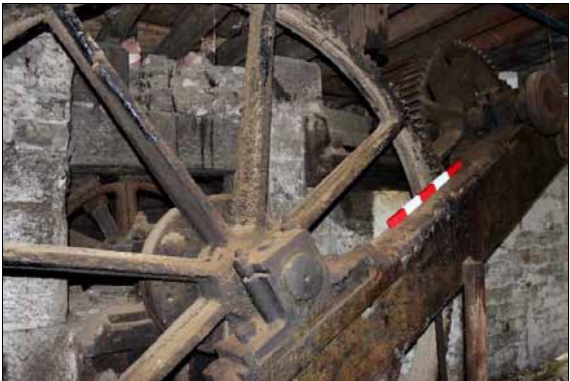
Plate 66: 8' gearing wheel on pinion wheel axle
