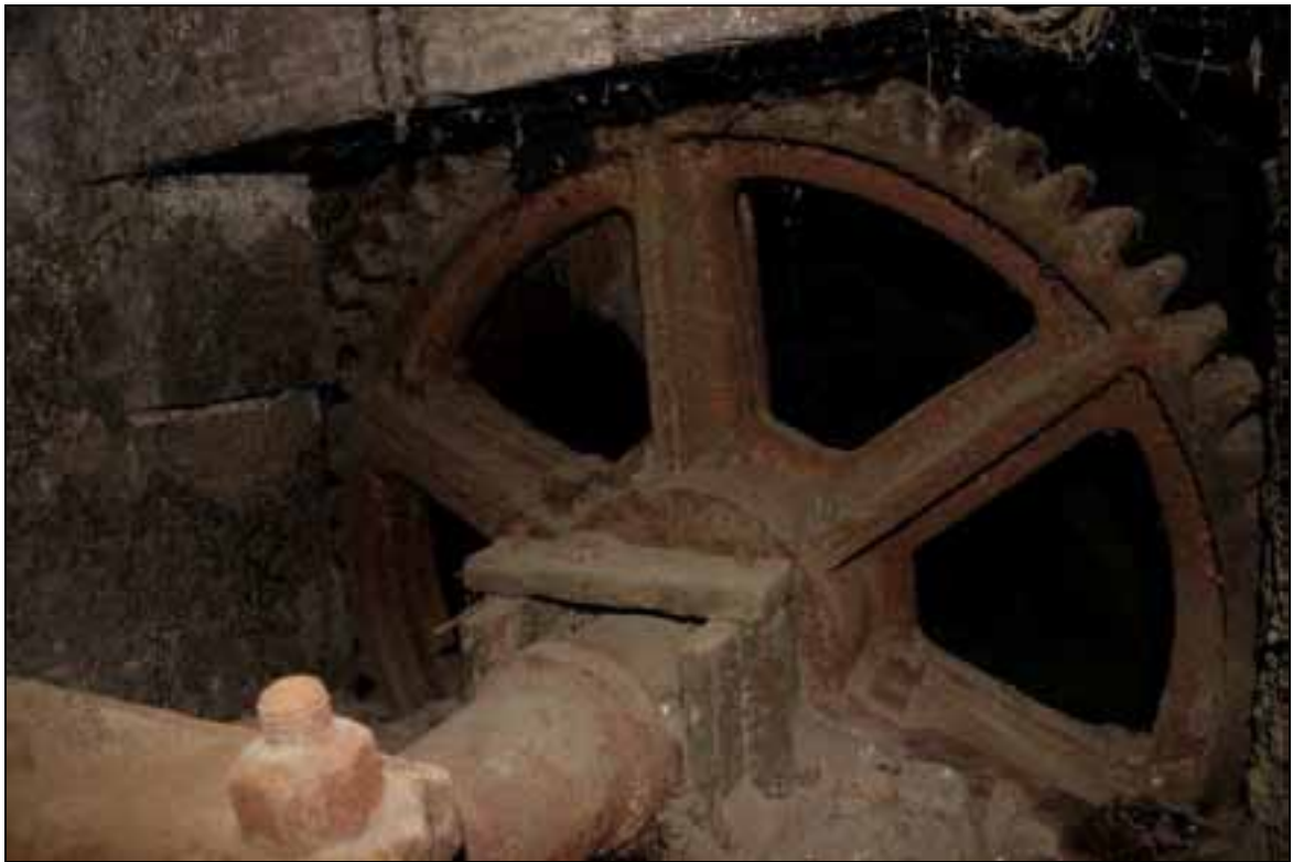
Plate 65: Axle and bearing of pinion wheel
