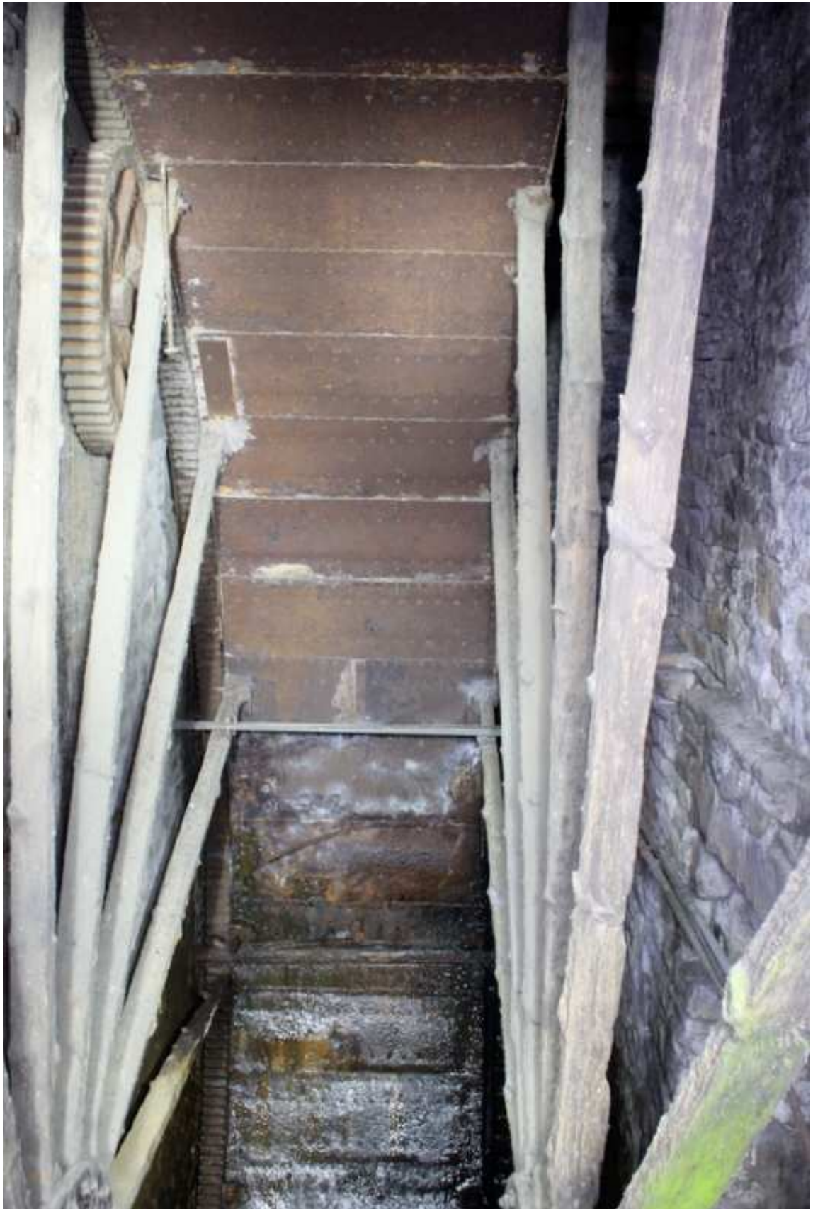
Plate 69: Extant waterwheel with slender timber spokes
