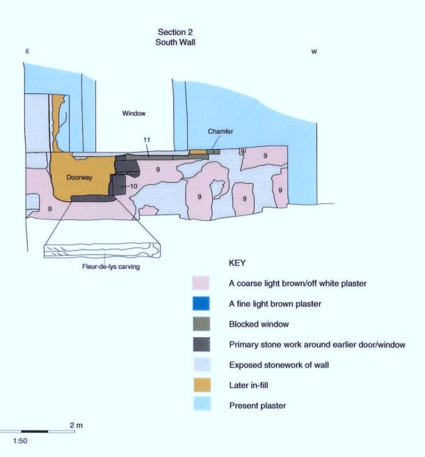
Figure 3: Elevations of north and south wall
