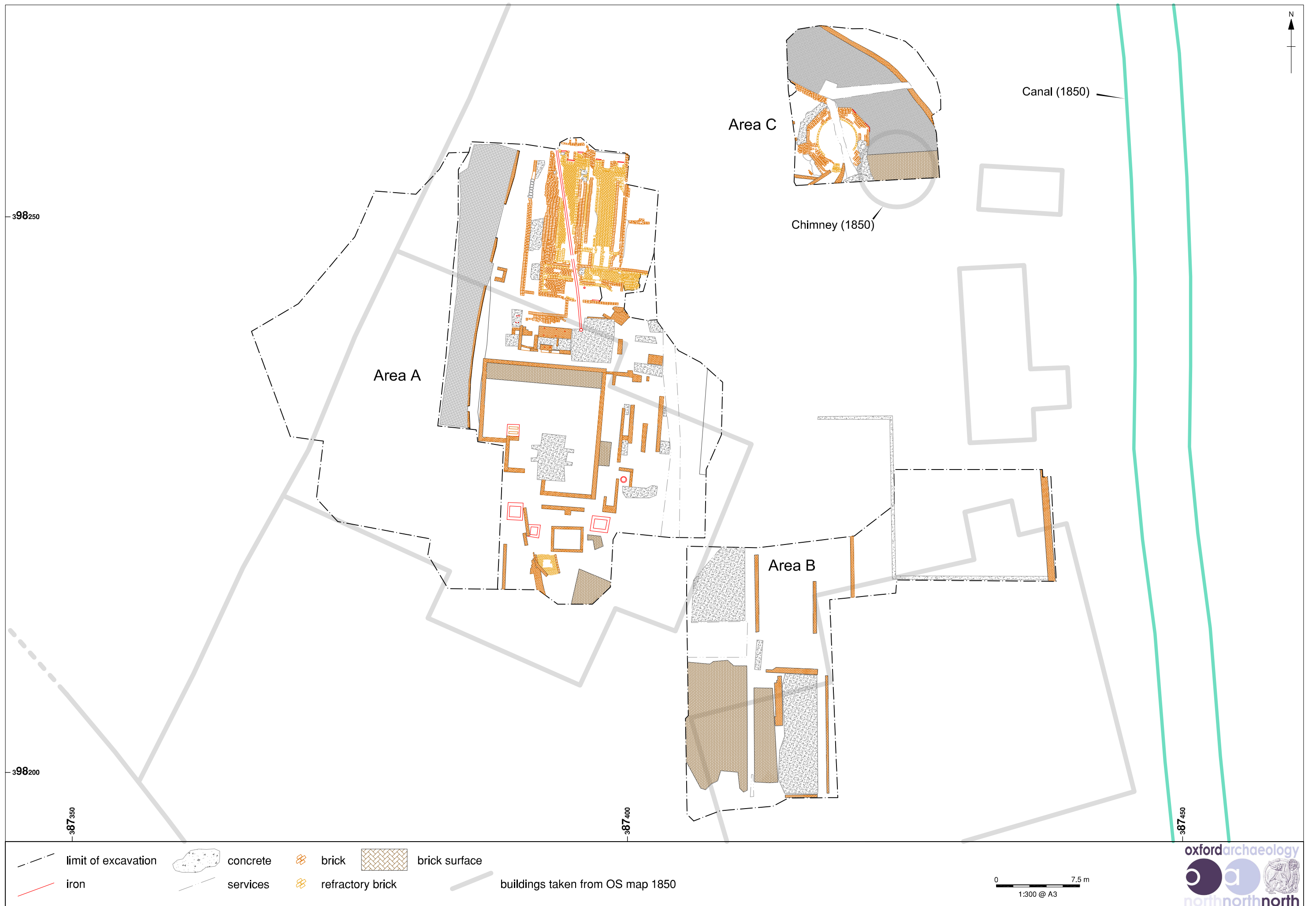
Figure 5: The excavated remains of Clayton Chemical Works
