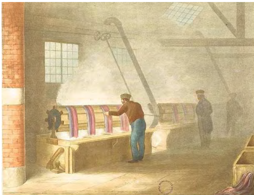
Plate 5: A mid-nineteenth-century engraving of the dyeing process (from Barfoot 1840)
