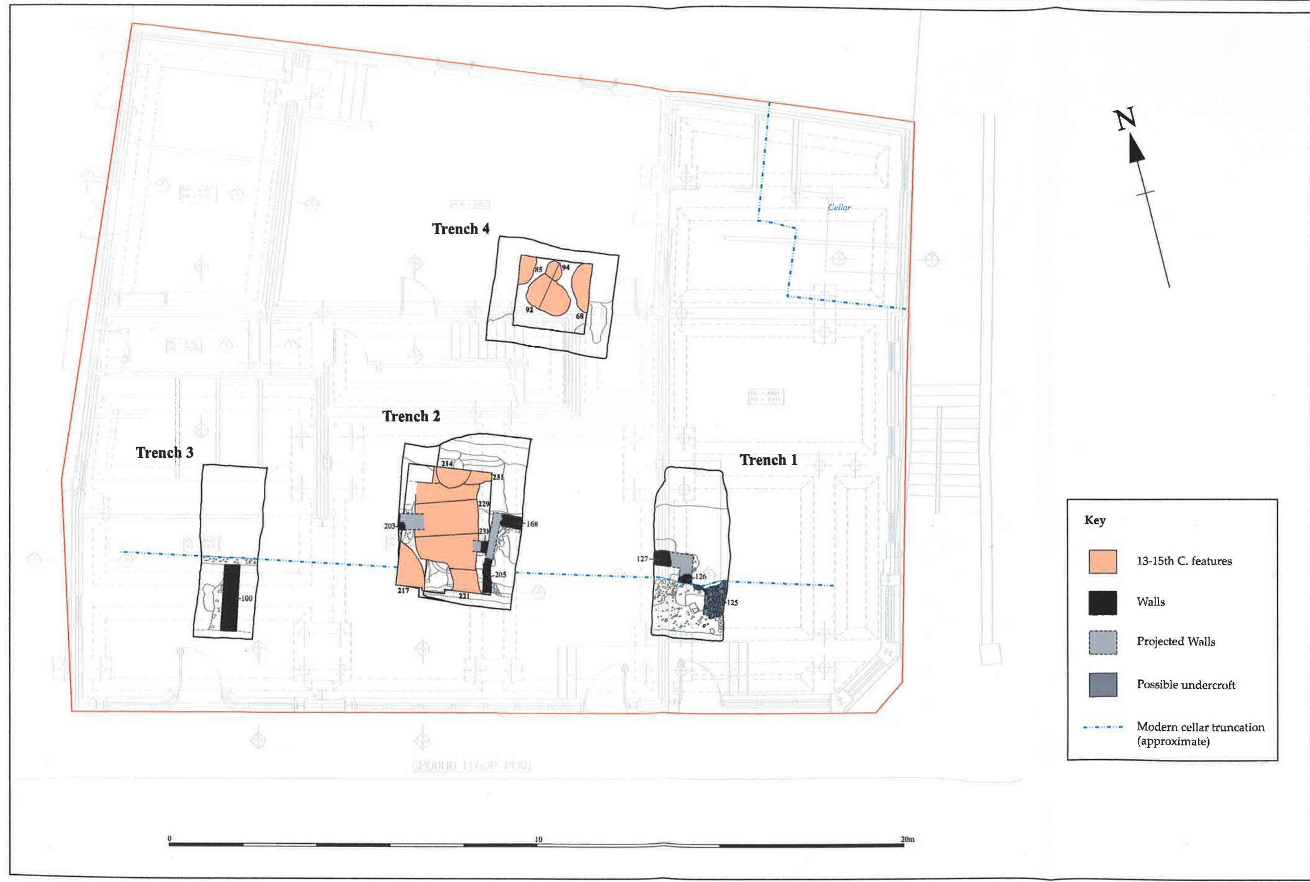
Figure 2: Evaluation trenches overlaid on ground plan of proposed building with principal features annotated
