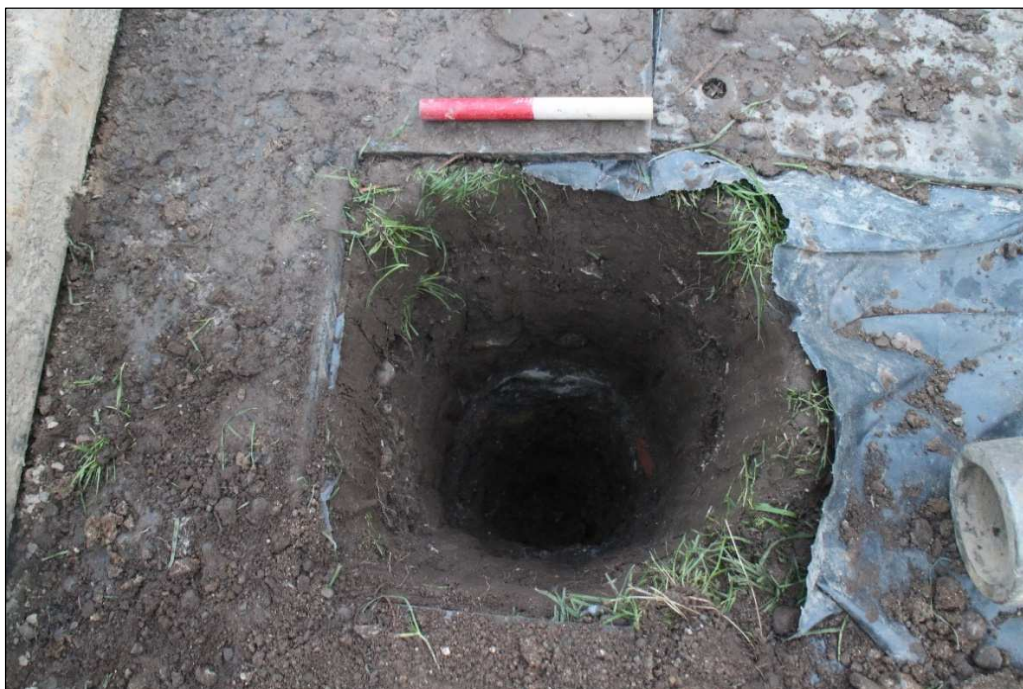
Plate 2: BHK28 showing limestone inclusion 2802 , scale 0.20m
