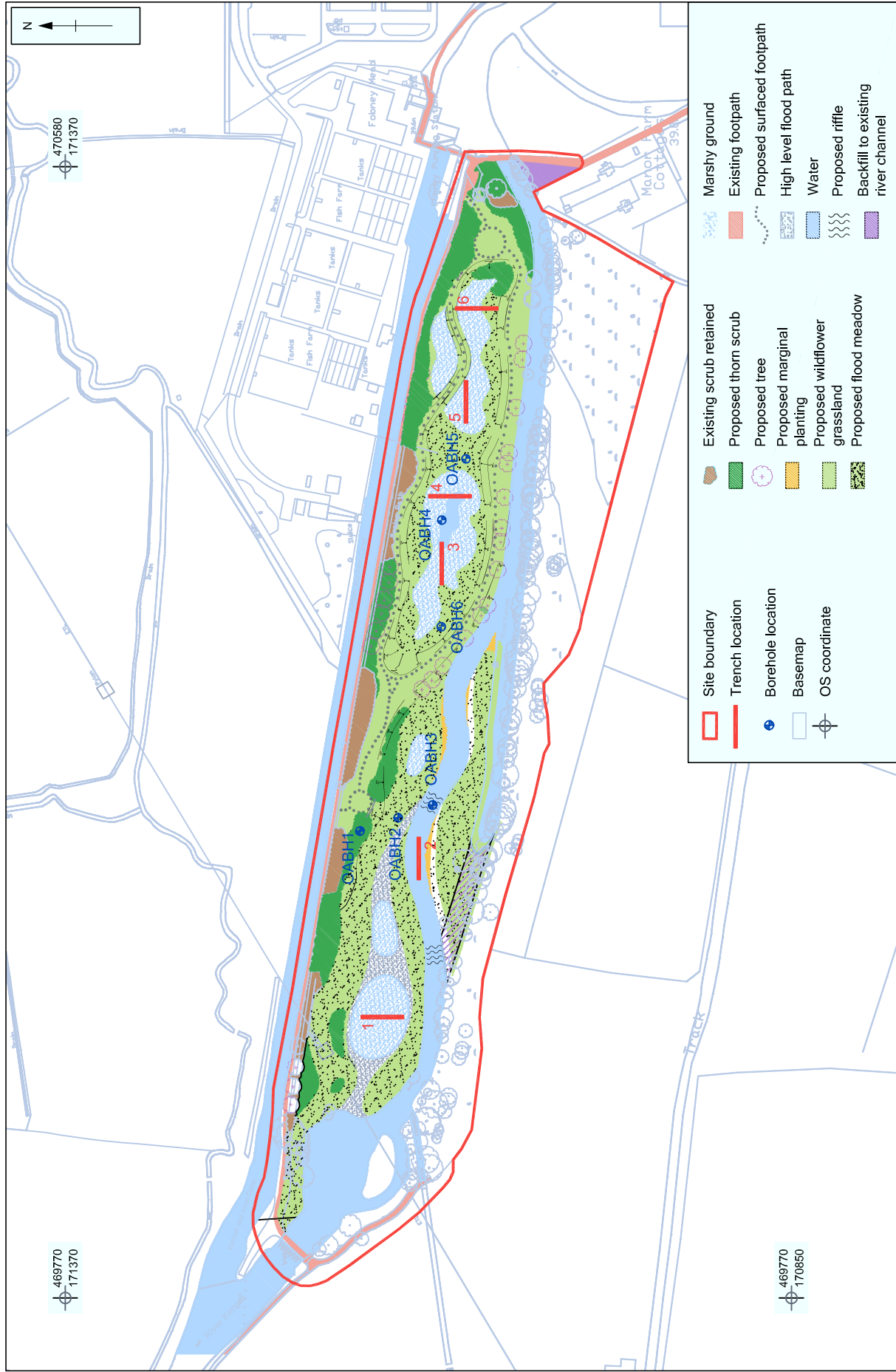
Figure 3: Trench and borehole locations
