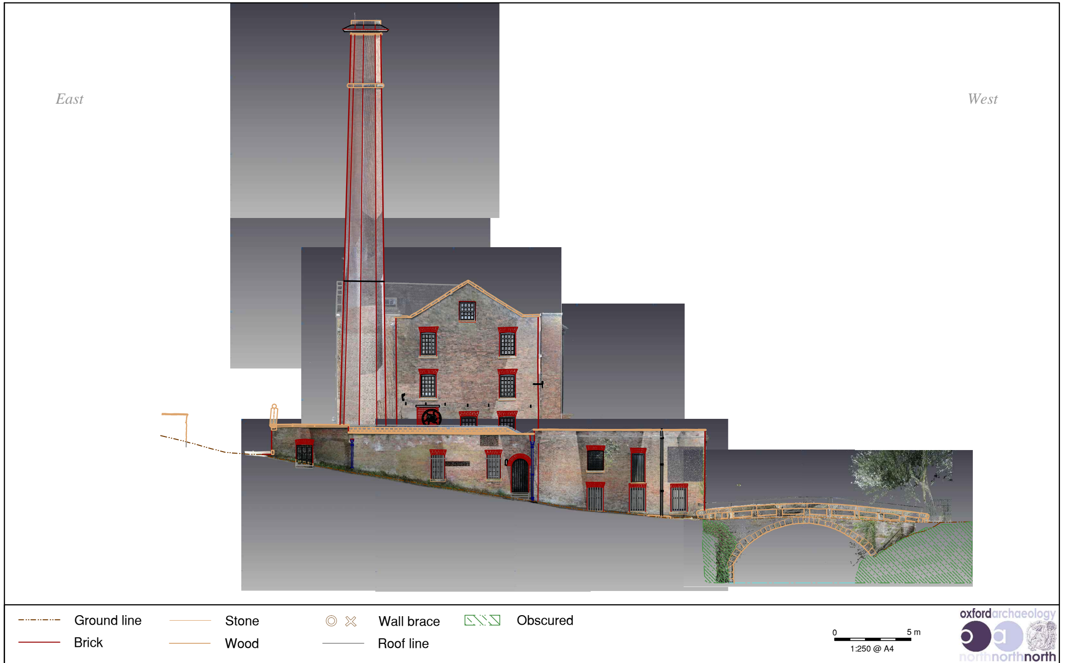
Figure 140: Elevation 2 - The Engine House and Old Mill Gable including Laser Scan data
