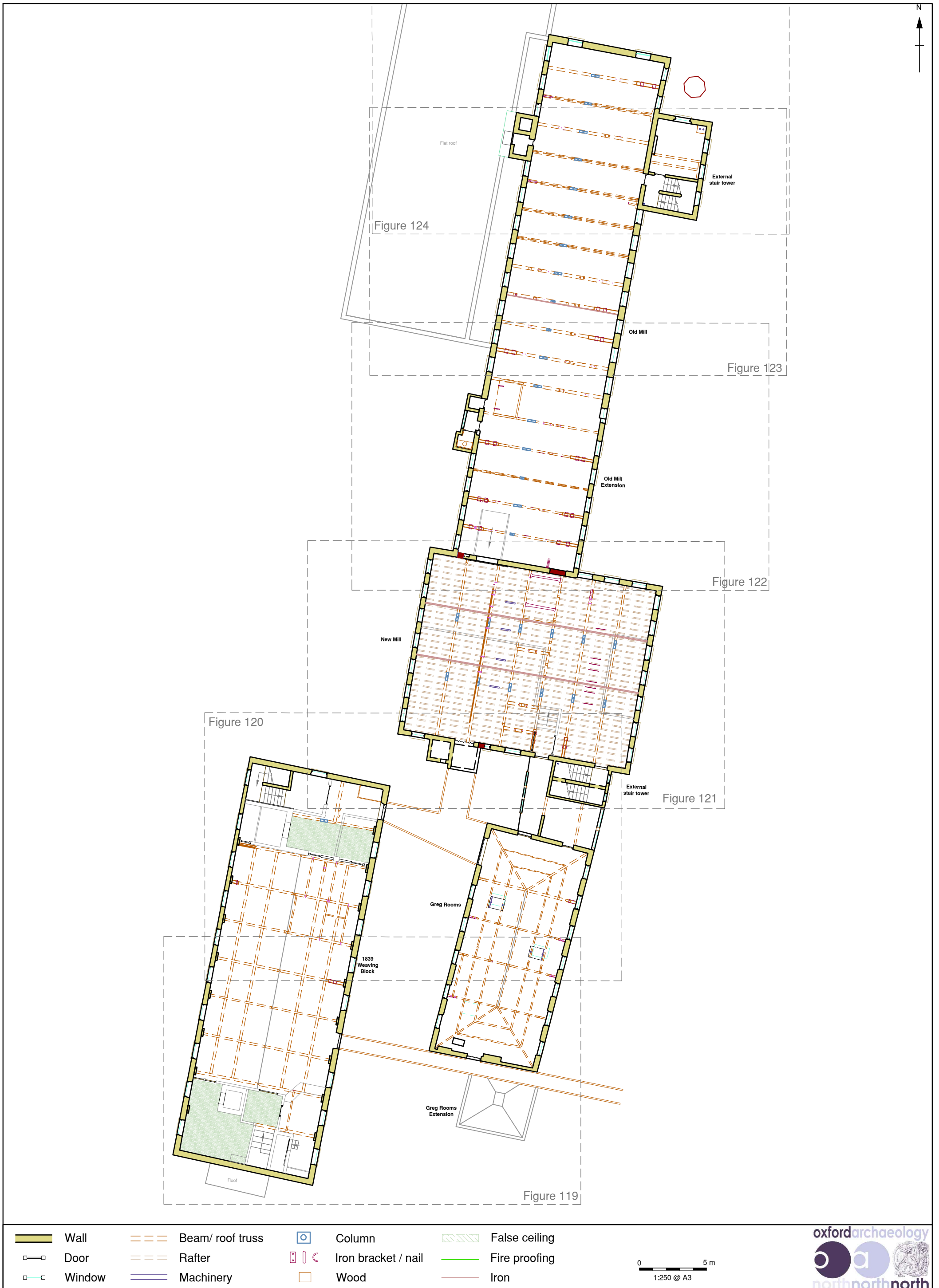
Figure 118: Quarry Bank Mill Overall Second Floor Plan
