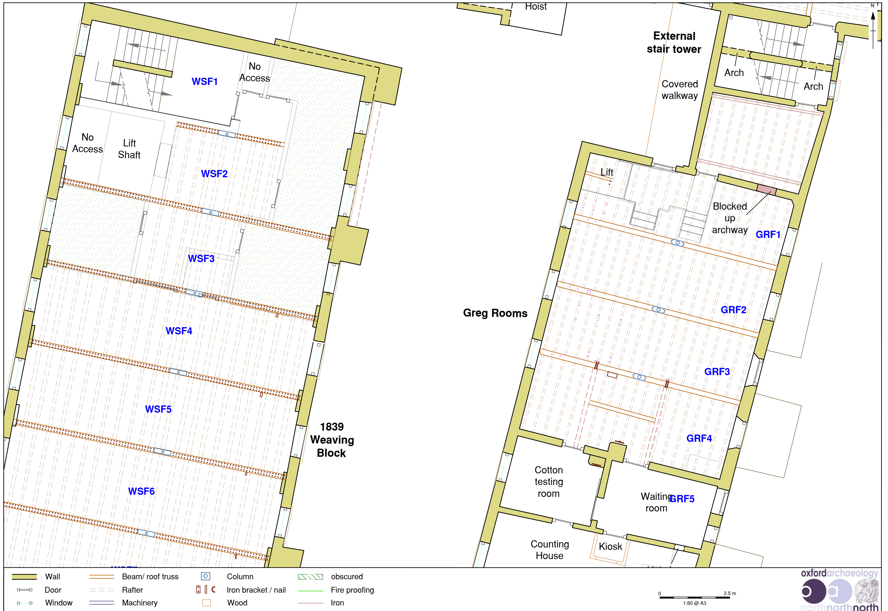
Figure 113: First Floor - 1839 Weaving Block and Greg Rooms (North)
