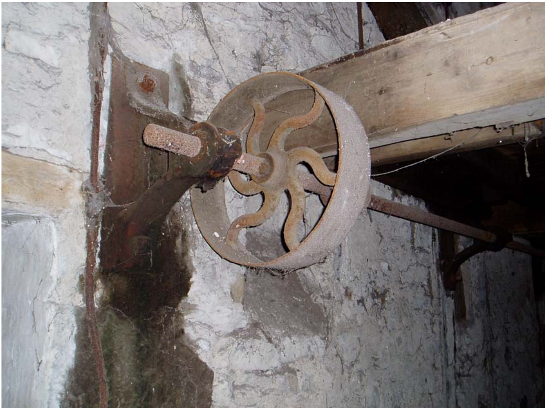
Plate 17: The spoked flywheel and lineshaft within the barn
