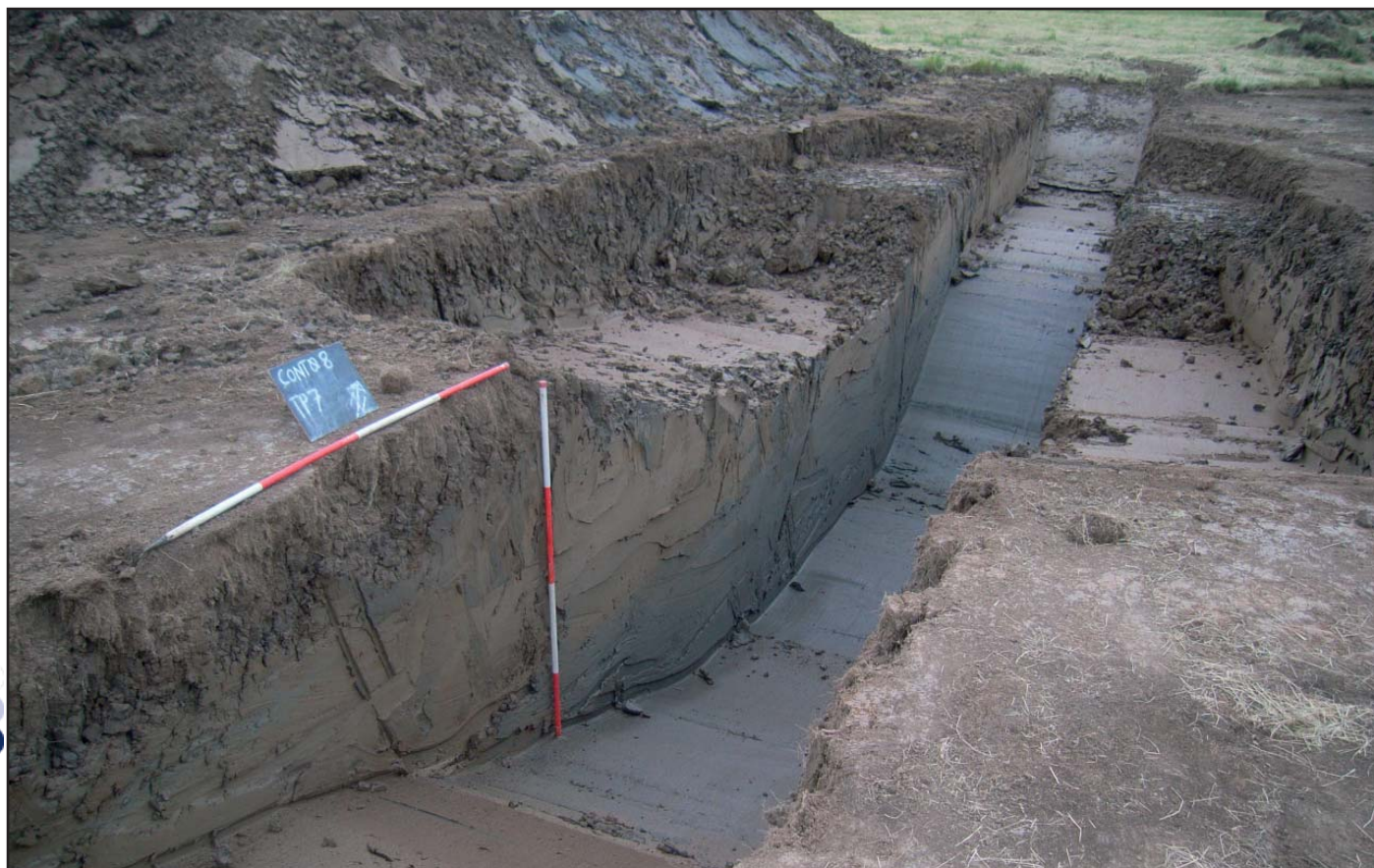
Figure 4: Trench 7, illustrating the relatively homogeneous upper alluvial stratigraphy in the Northern Triangle: In general the sequence comprised a grey brown silty A horizon with prismatic structure, under which was a grey brown clay silt with Fe mottling, underlain by a blue grey silt clay to the base of excavation.
