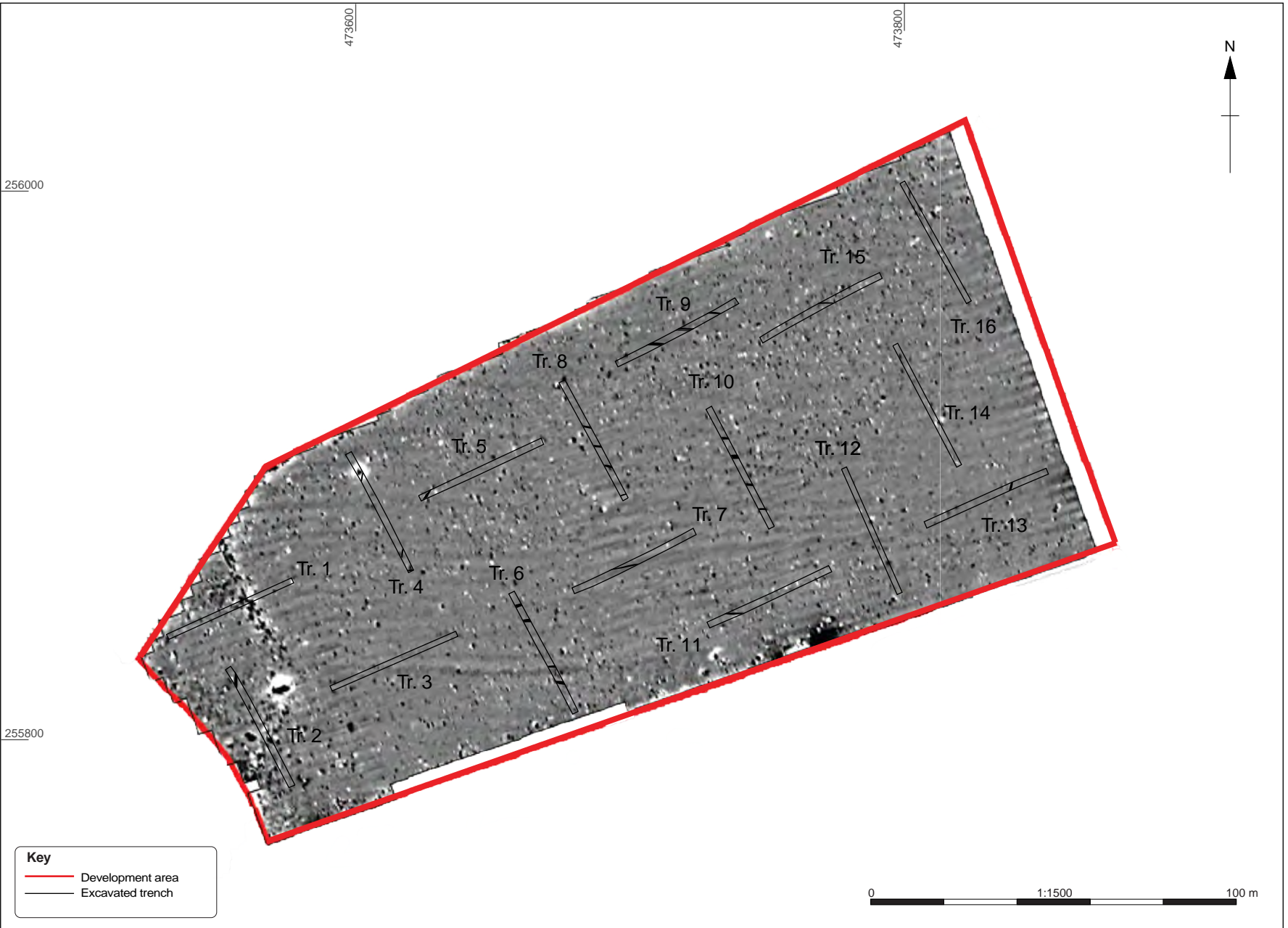
Figure 4: Trench plan overlain of geophysical survey results
