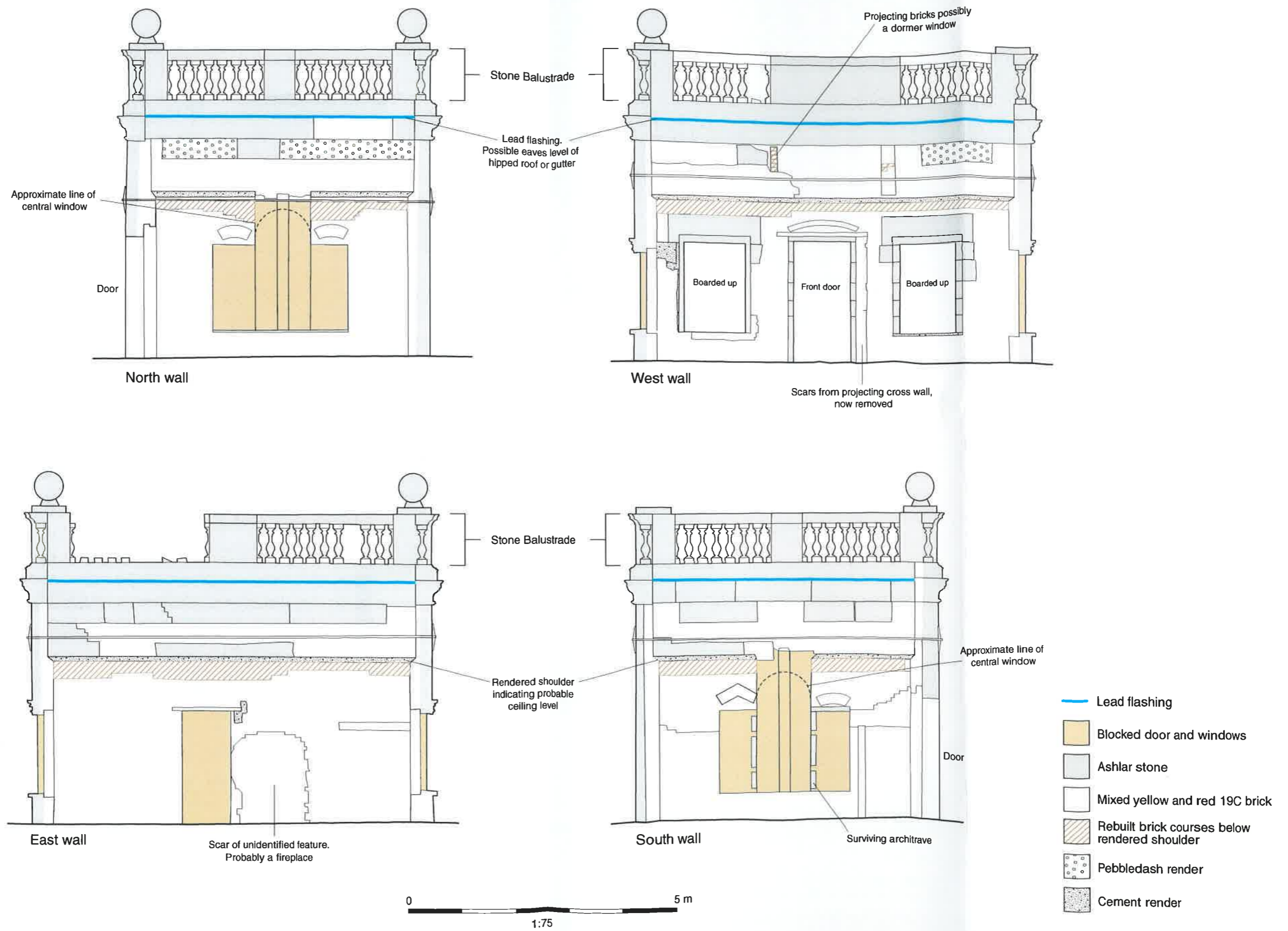
Figure 11: Temple Bar, interior Lodge elevations
