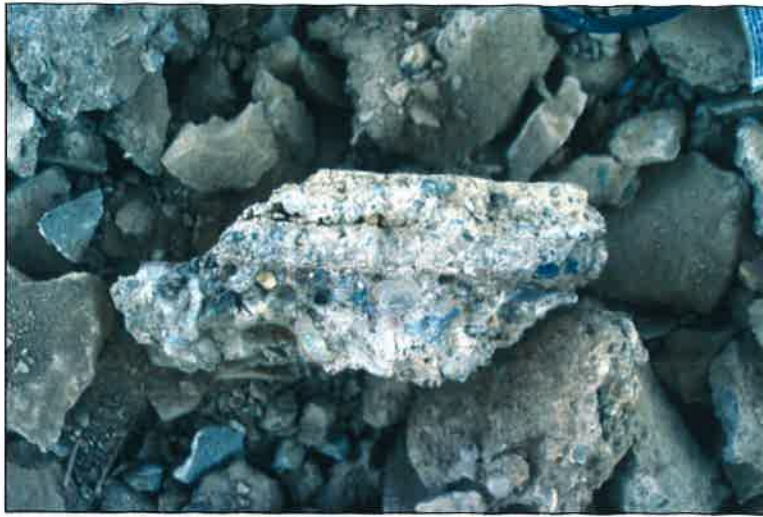
Plate 27: Section of concrete, showing the three layers making up the floor inside the upper room (OA 2004, F8/04)
