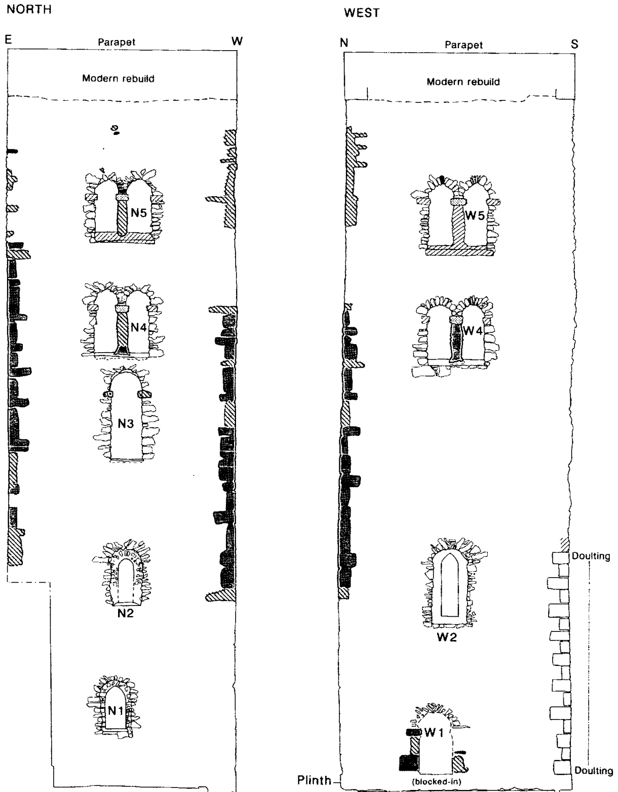
Figure 4.14 St Michael's Church Tower: north and west elevations showing detail of stone. Scale as Fig. 4.15.
