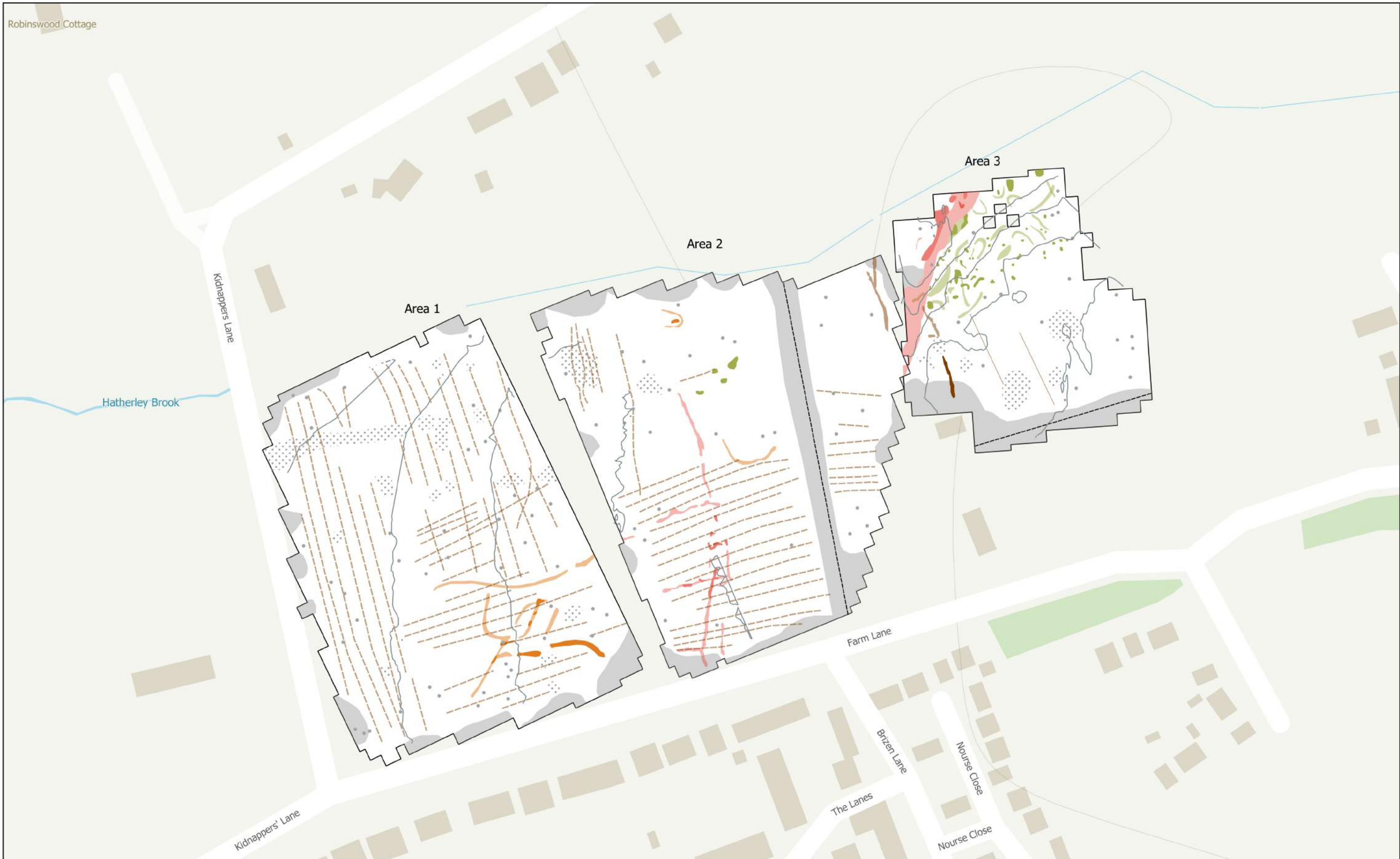
MSSO490 - Farm Lane, Cheltenham Figure 4 - Magnetic Interpretation with contours 1:1,500 @ A3 Copyright Magnitude Surveys Ltd 2019 Contains Ordnance Survey data © Crown Copyright and database right 2019)
