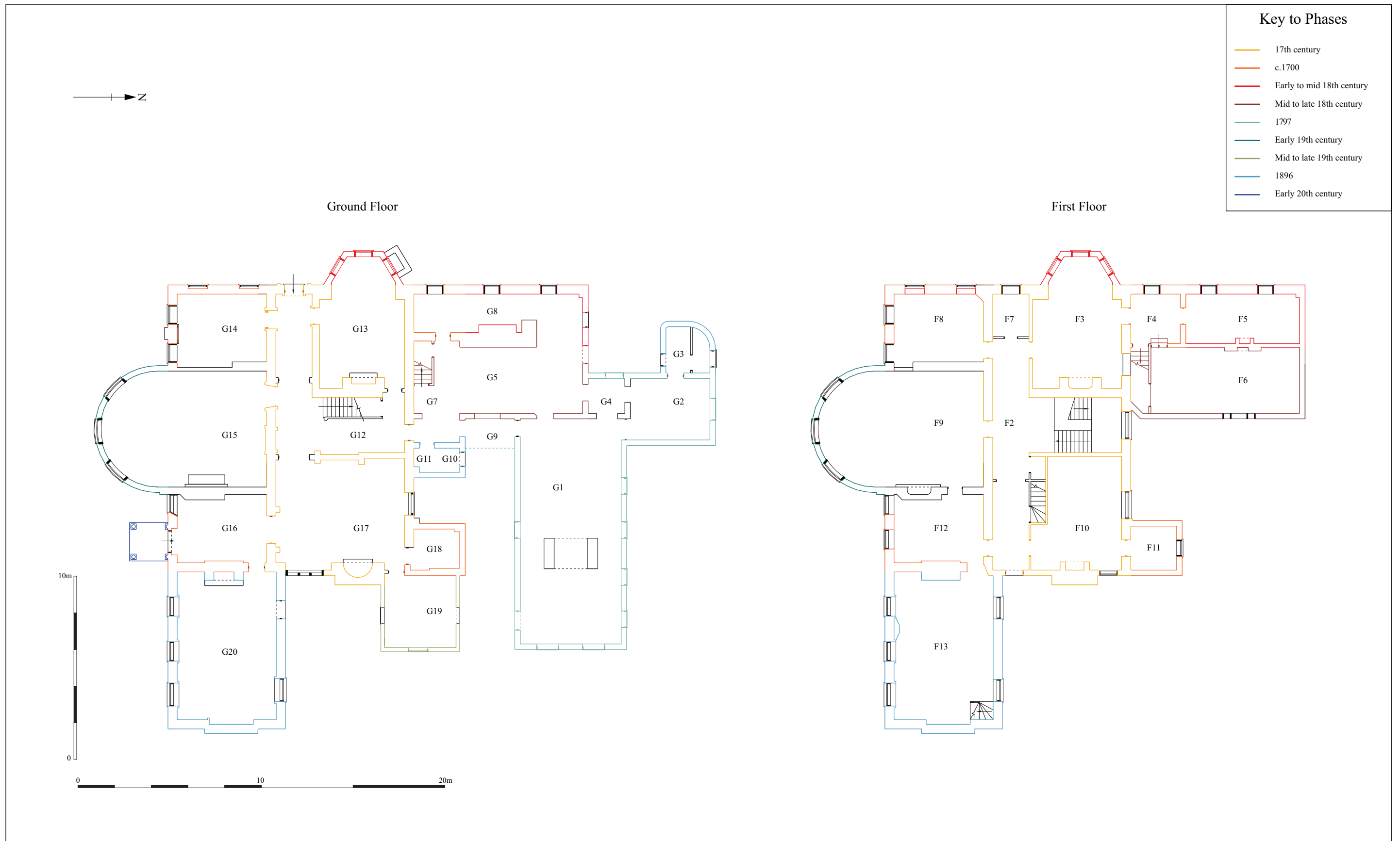
Figure 10: Ground and first floor plans (with phasing), Orford House (reproduced from data supplied by Lowden Construction)
