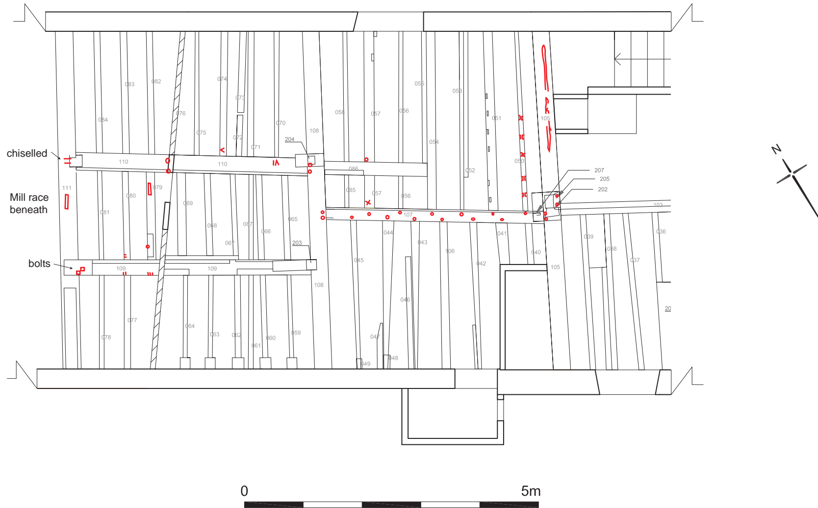
Figure 5: Plan of joists in western half of ground floor (from MOLA study) showing carpenters' marks, pegs and other features on top of joists recently exposed by removal of floorboards
