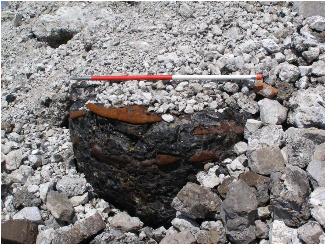
Plate/Shot 20: Detailed view of blast furnace slag at the south end of site, looking north-west
