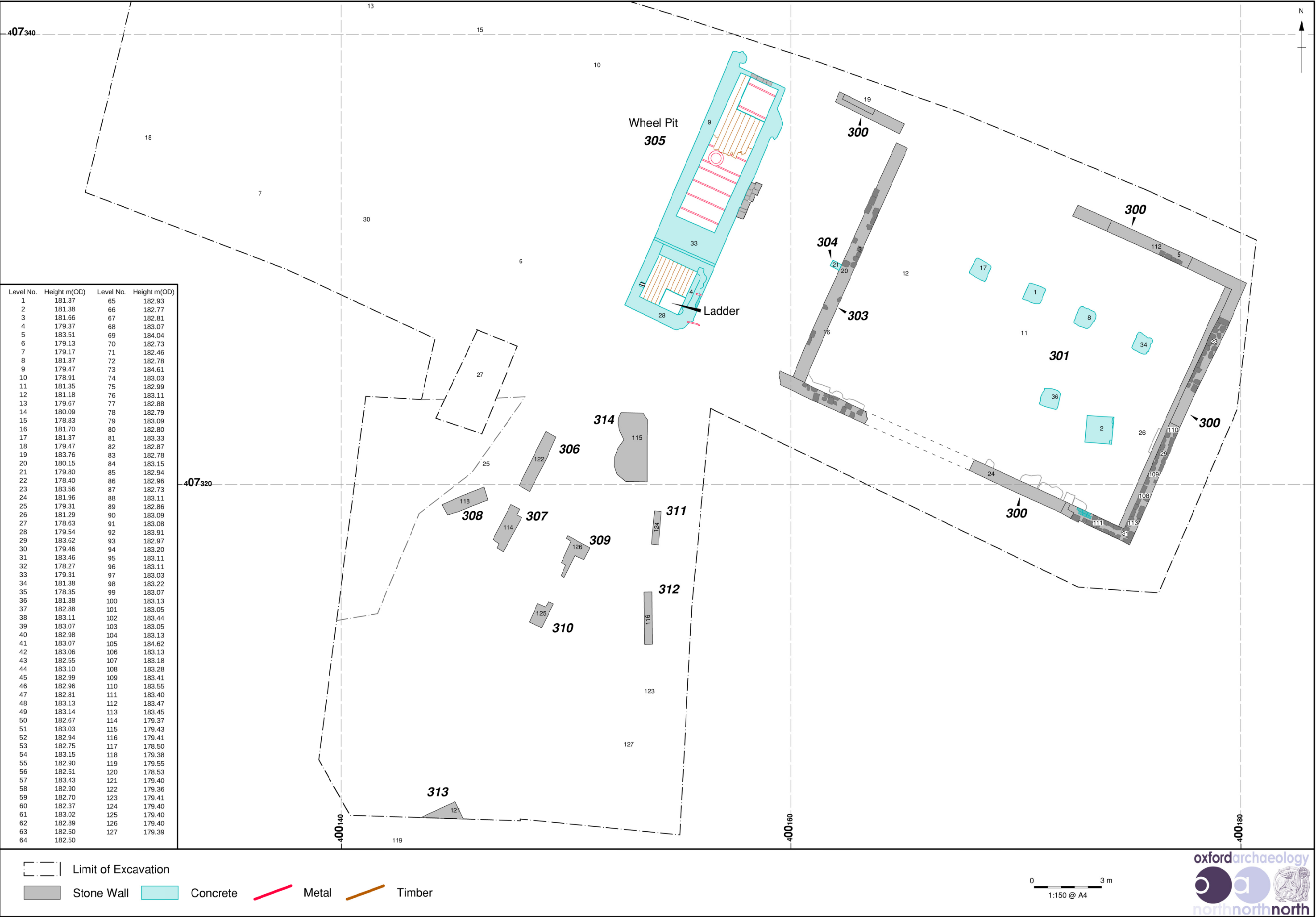
Figure 6: The remains exposed during the strip, map and record of Wrigley Mill, Area 3
