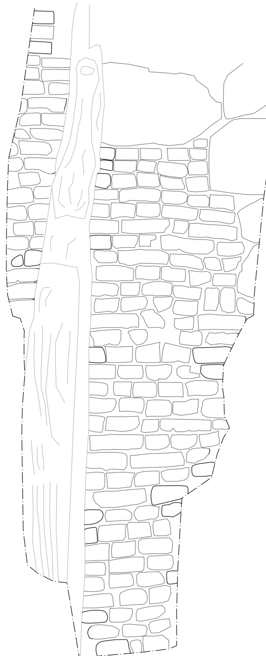
Figure 15 North-Facing Elevation of Dock Wall in Trench 7
