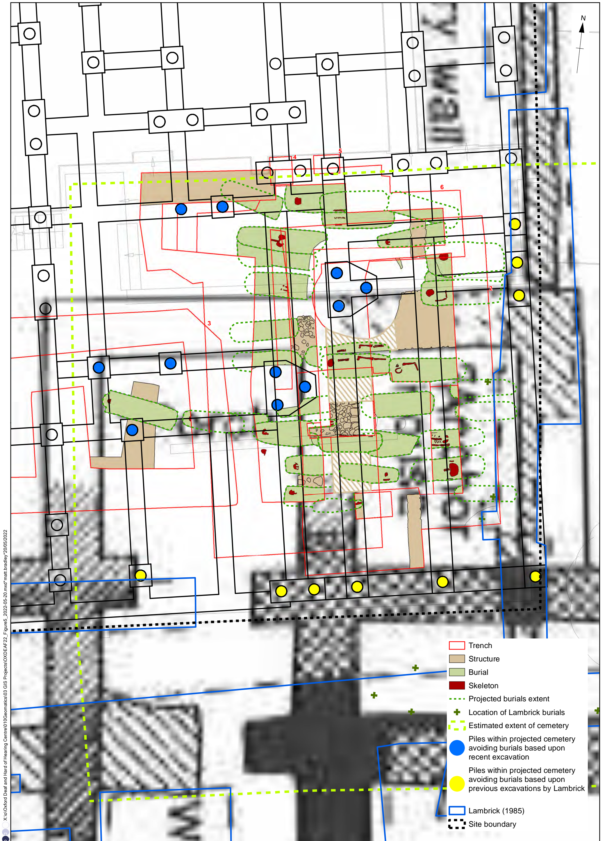
Figure 5: Showing revised foundation design and position of piles to avoid burials with projected cemetery
