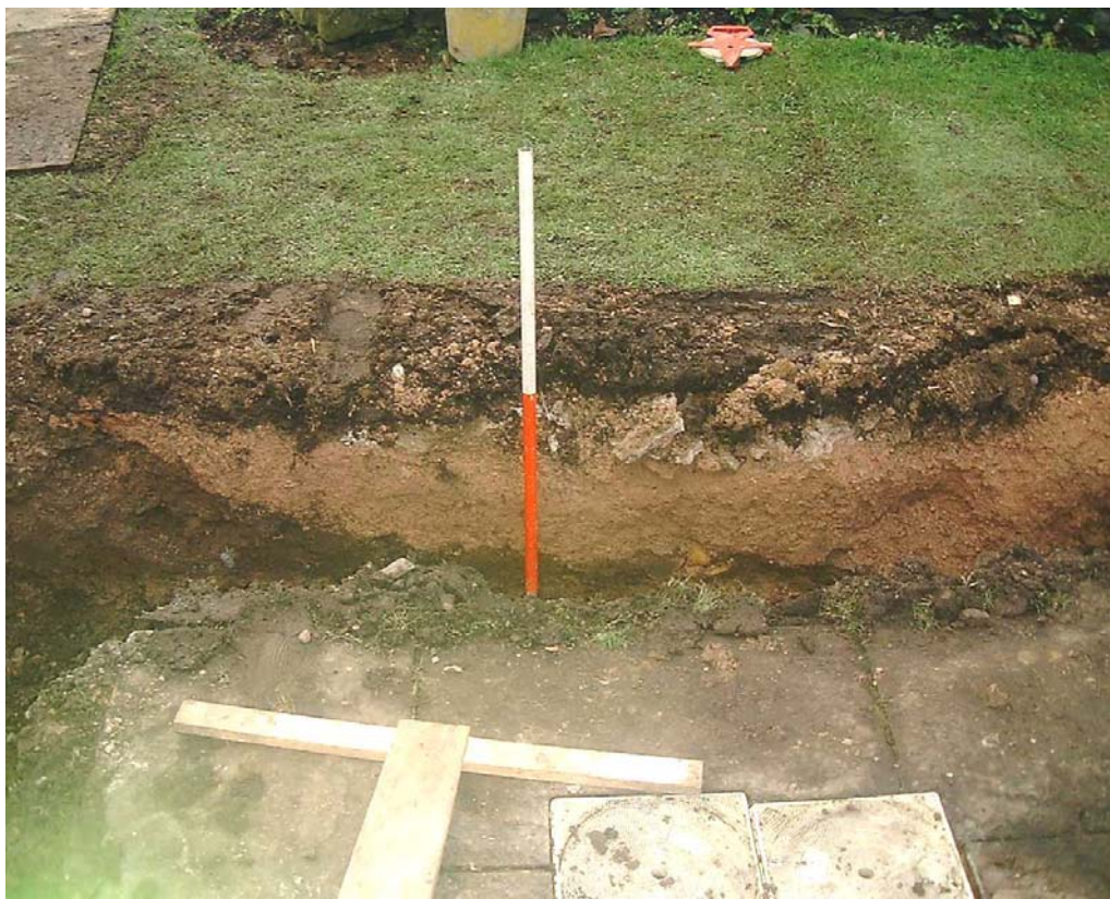
Plate 5: Section to the South of the Swimming Pool Showing Hardcore
