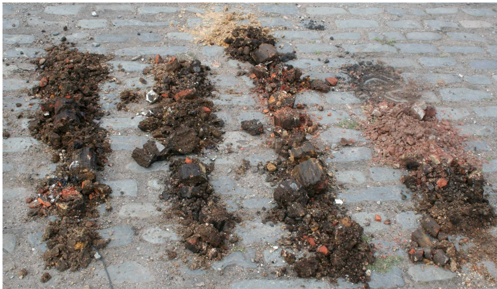
Plate 4: Risings from Window Sample Bore Hole WS104 demonstrating the mixture of industrial and domestic waste used to backfill the abandoned quarry seams
