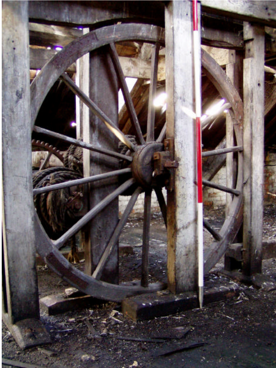
Plate 25: Detailed Shot of Winch Mechanism in Room 22.TF1
