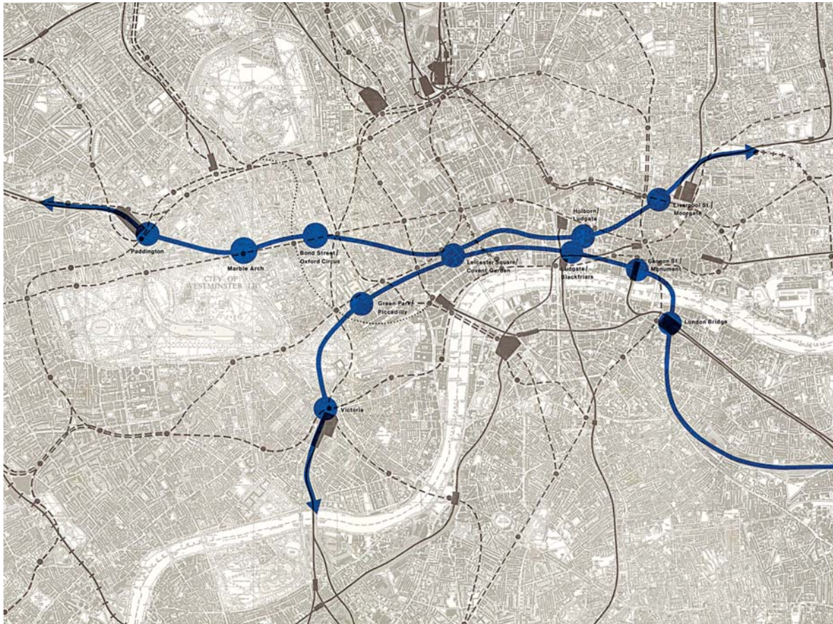
Fig 127 The 1974 London Rail Study advocated new tunnels to connect British Rail’s Western Region with its Eastern Region, and Victoria station with London Bridge (Crossrail)
