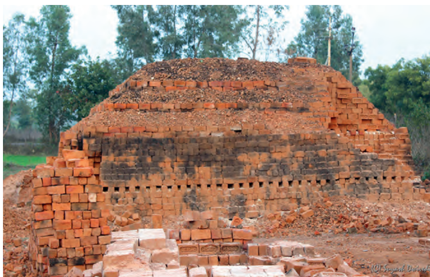
Fig 40 (right) A brick clamp in present day India (Suyash Dwivedi, CC BY-SA 4.0)
