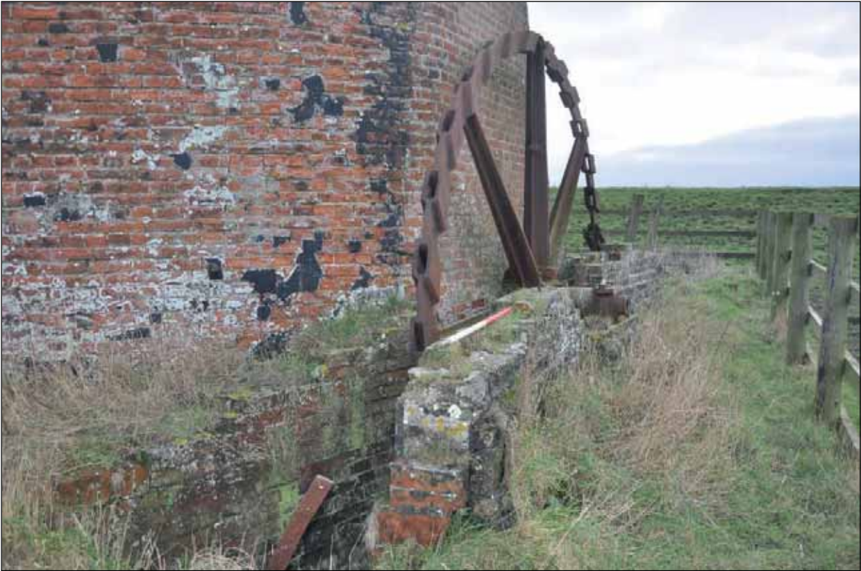
Plate 23: Iron linking gear and wheel within remains of scoopwheel housing, from the north-west
