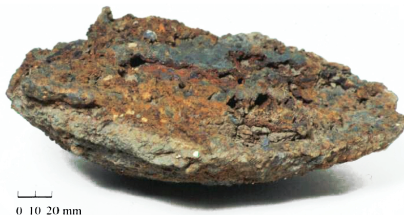
Plate 7.3 Furnace bottom slag from the side (circular in plan).
