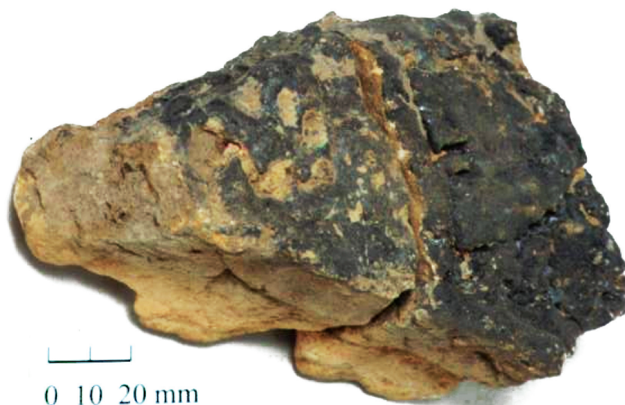
Plate 7.1 Wedge-shaped fragment of slag-coated clay, with a flat edge at the bottom of the picture, a reasonably flat edge at the top of the picture and the point of the wedge in the foreground.
