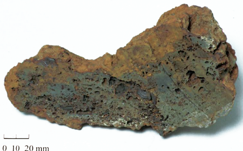
Plate 7.4 Cross section of large smithing hearth slag.
