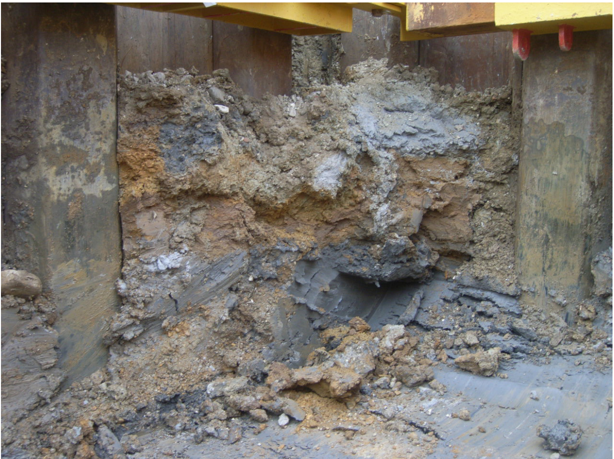
Plate 8: Fluvial channel fills overlying London Clay at the northern end of the thrust pit
