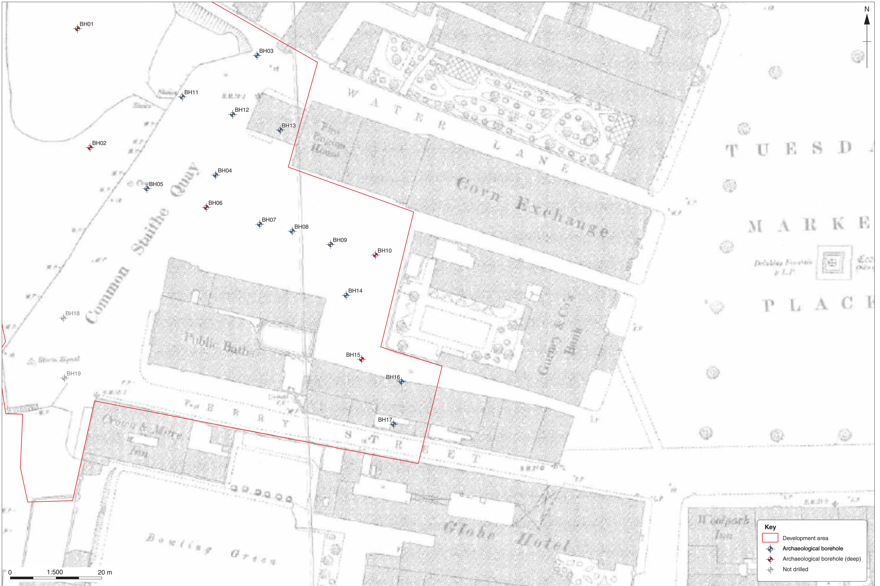
Figure 5: Borehole array with the 1883 Ordnance Survey plan, Common Staithe. Scale 1:500 at A3
