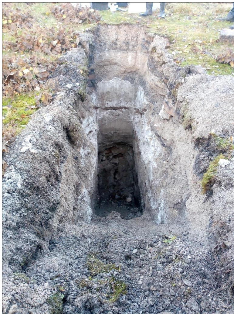
Plate 3: TP 08 showing brickwork at the base, and in the top right-hand side
